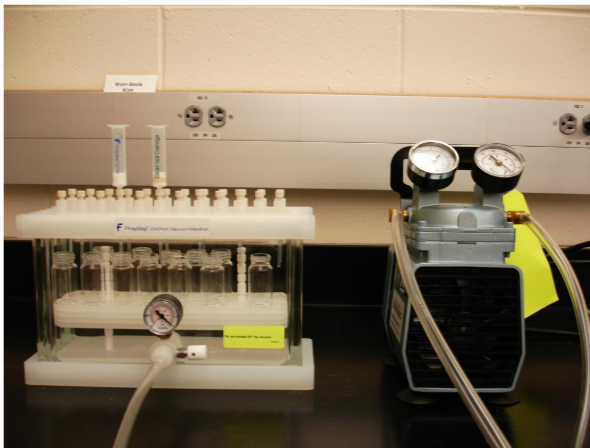
Figure 3.2. Extraction manifold (vacuum manifold) and pump
