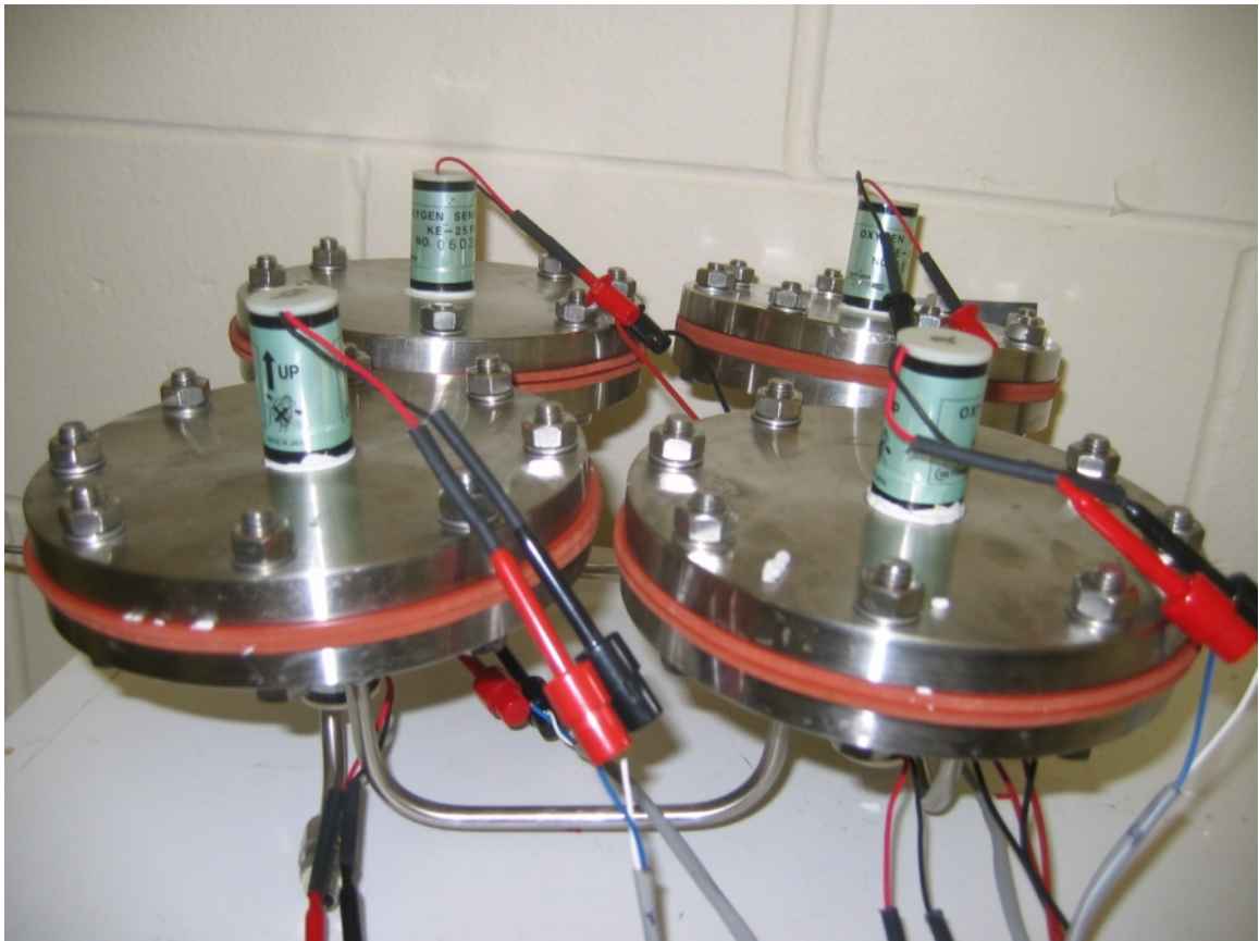
Figure 3-6 Test Specimens Set Up – 1 Control and 3 Test Cells
