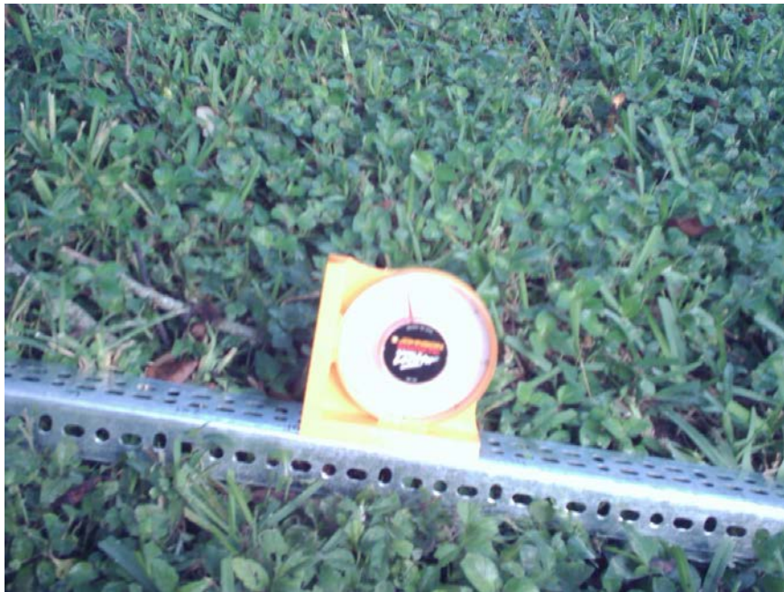
Figure 4.6: Field instrument to measure inclination angle of roadside slopes
