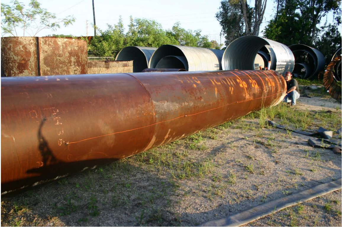
Figure 3-5: Voided Shaft Thermocouples on Outside of Central Casing.
