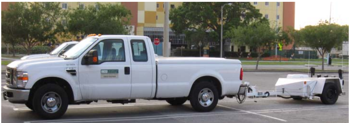
Figure A.2: Locked Wheel Skid Tester (LWST)
