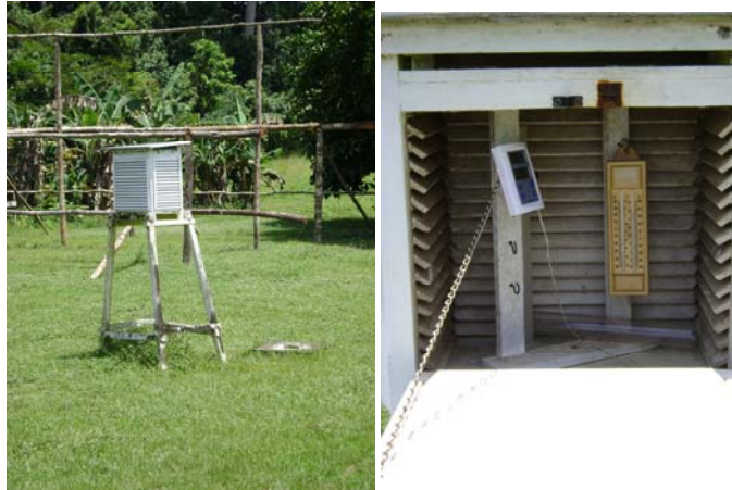
Figure C18 Weather station external (left) and internal (right).
