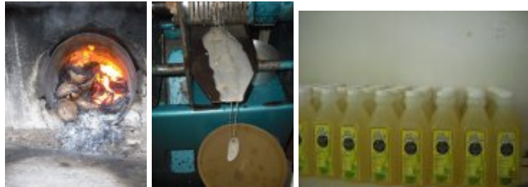
Figure C31 Stages of JamOrganiX's coconut oil production. Left through right: Drying of shredded coconut; pressing of dried coconut and filtering of oil; bottling of final product.
