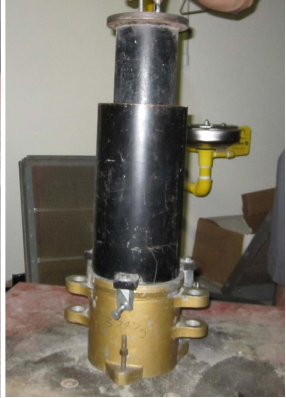
Figure 4.5: Placing Weight in Sleeve
