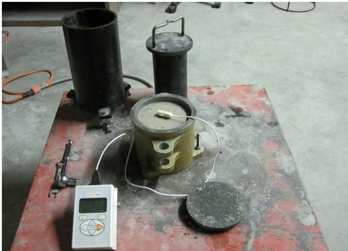
Figure 4.3: Performing Thermal Conductivity Test on Non-compacted Soil
