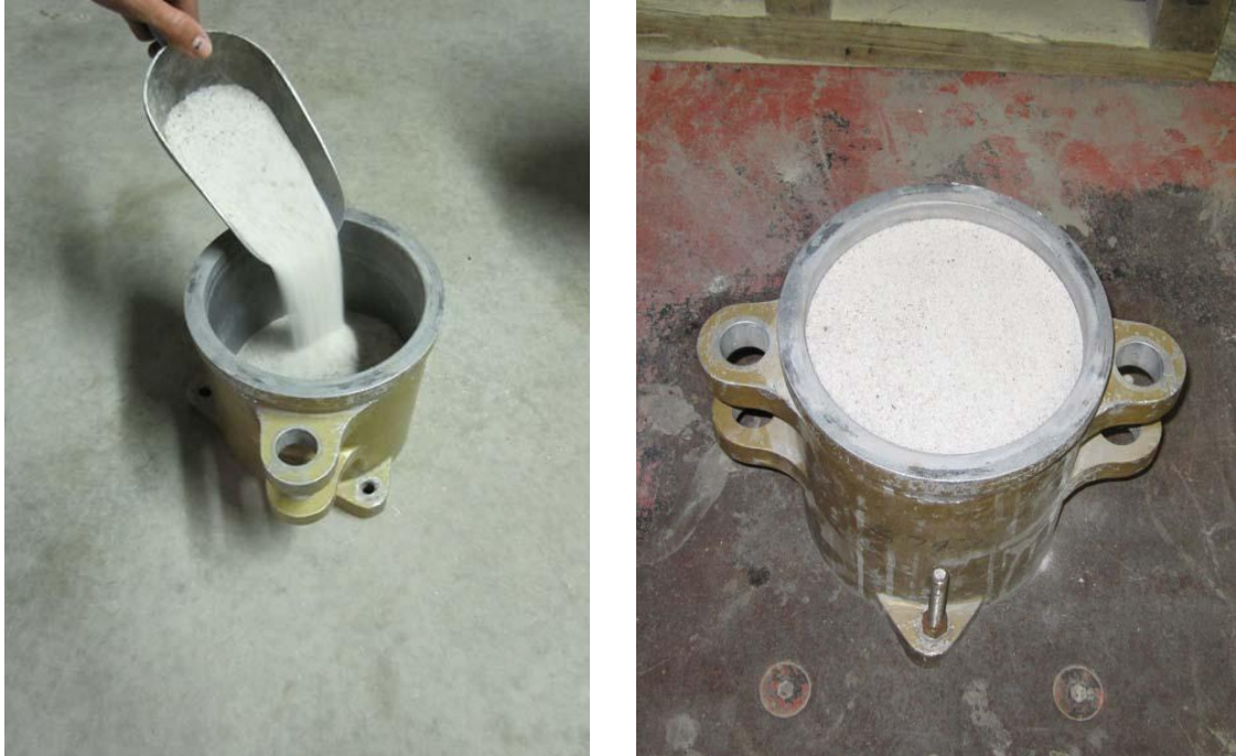
Figure 4.2: Placing Sand into Mold and Attaching it to the Vibrating Table
