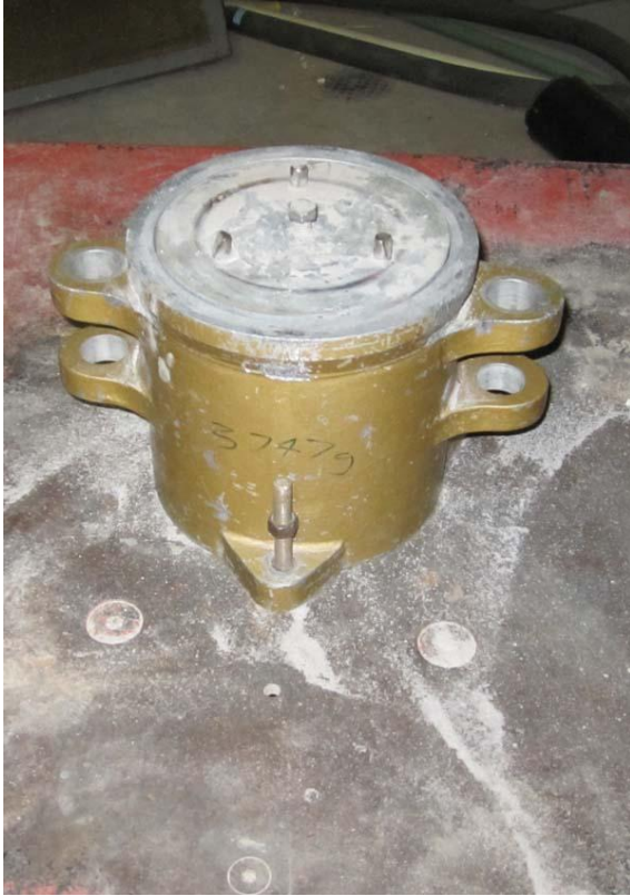
Figure 4.4: Baseplate Placed on Mold
