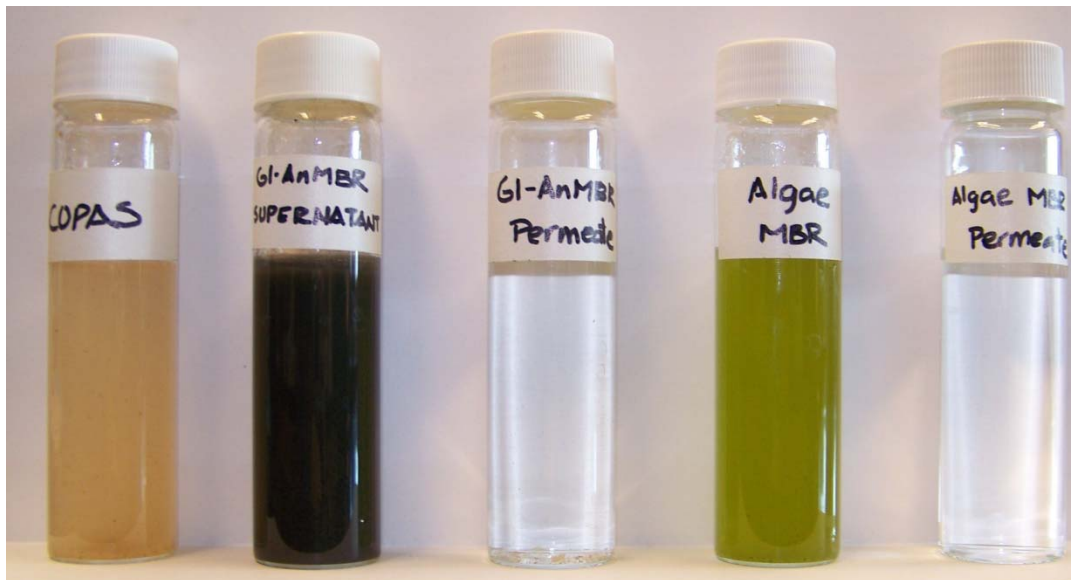
Figure 7.1: Waste to Water in the A2MBR. From left to right: COPAS synthetic sewage, GI-AnMBR sludge, GI-AnMBR permeate, Gas lift APMBR mixed liquor and APMBR permeate and final product.
