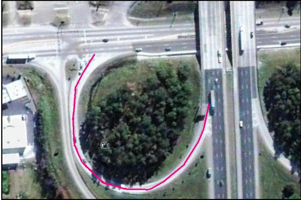
Figure 10-C. Free-flow Loop Exit Ramp Segment Length
