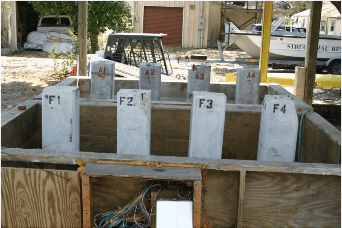
Figure 1.3 Test Piles in the Tank Awaiting FRP Wrap
