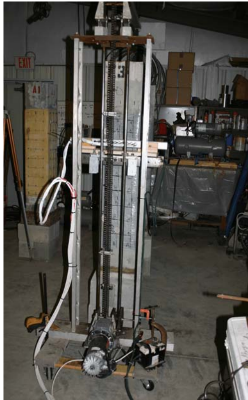
Figure 4.9 DEIT System Scanning a Pile
