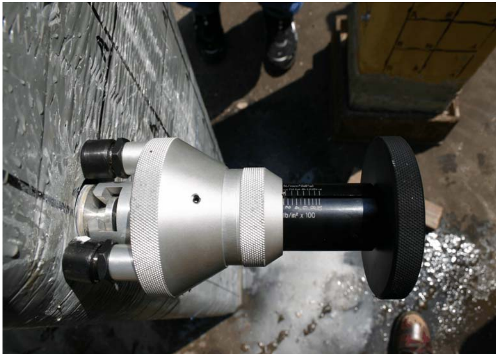
Figure 4.4 Elcometer Attached to Dolly for Pull-off Test
