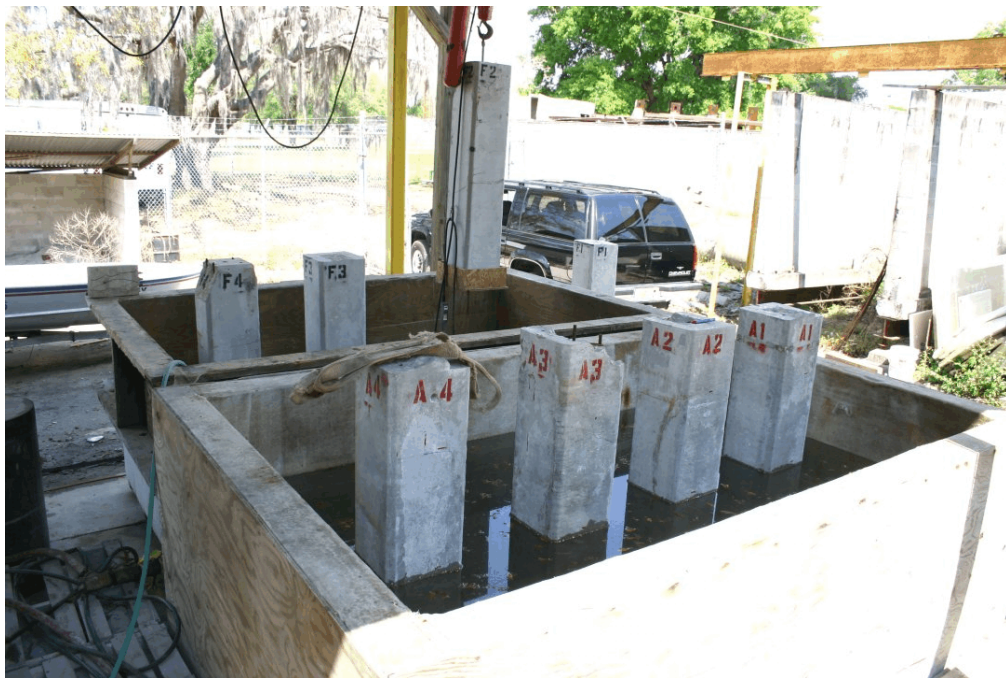
Figure 3.6 Piles in Tank, Awaiting FRP Application
