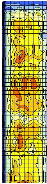
Figure C.107 Pile A4 Face C Thermal Scan
