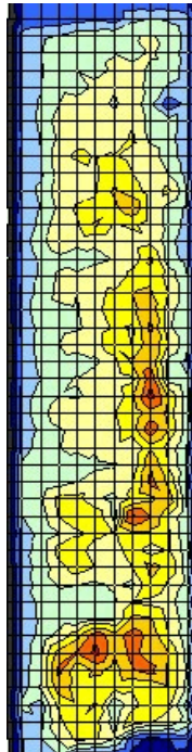
Figure C.64 Pile F4 Face D Thermal Scan
