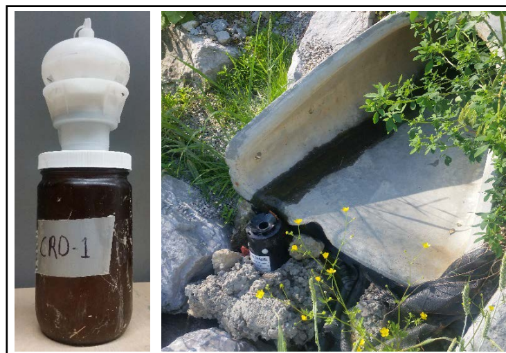
Figure 5: left—first flush jar; right—housing in rock apron
