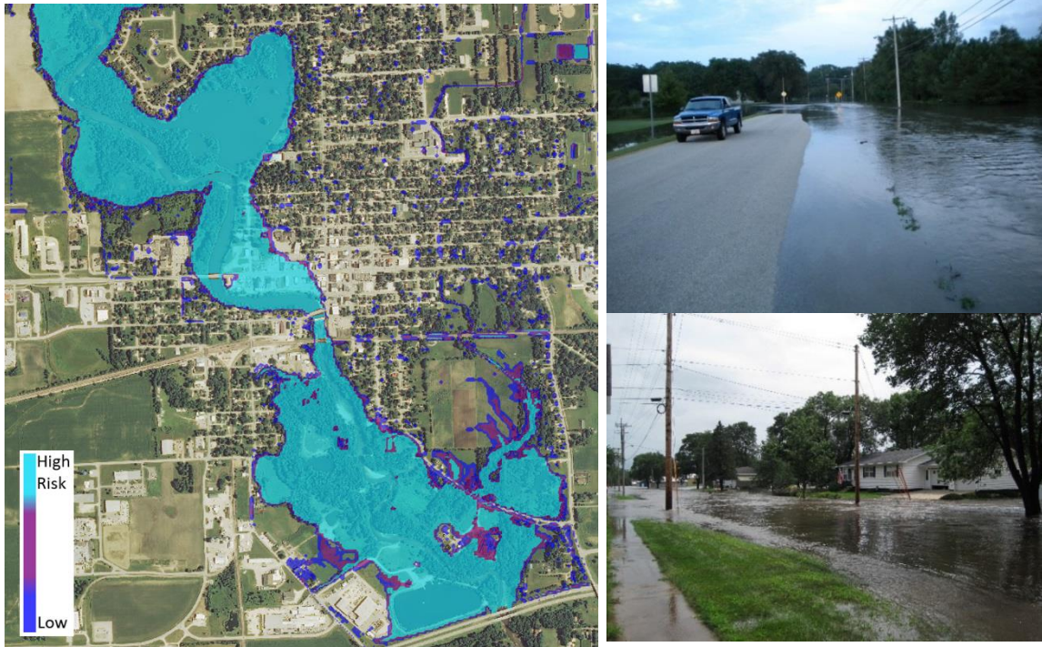
Figure 45. XP-C2 IFC max road safety risk for the July 2010 event compared to photos
