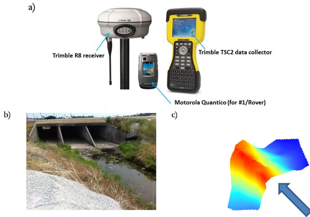
Figure 3.12 Real-time kinematic: a) components; b) testing location; c) mapping result
