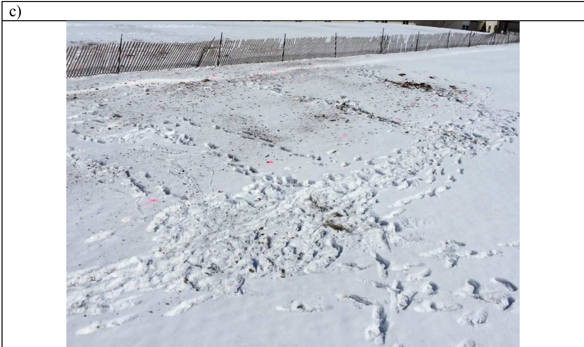
Figure 4.28 Seeding used for supporting the photogrammetric survey: a) instruments used to conduct the seeding (power generator and leave blower); b) view of upwind area of the snow fence; c) view of downwind area of the snow fence
