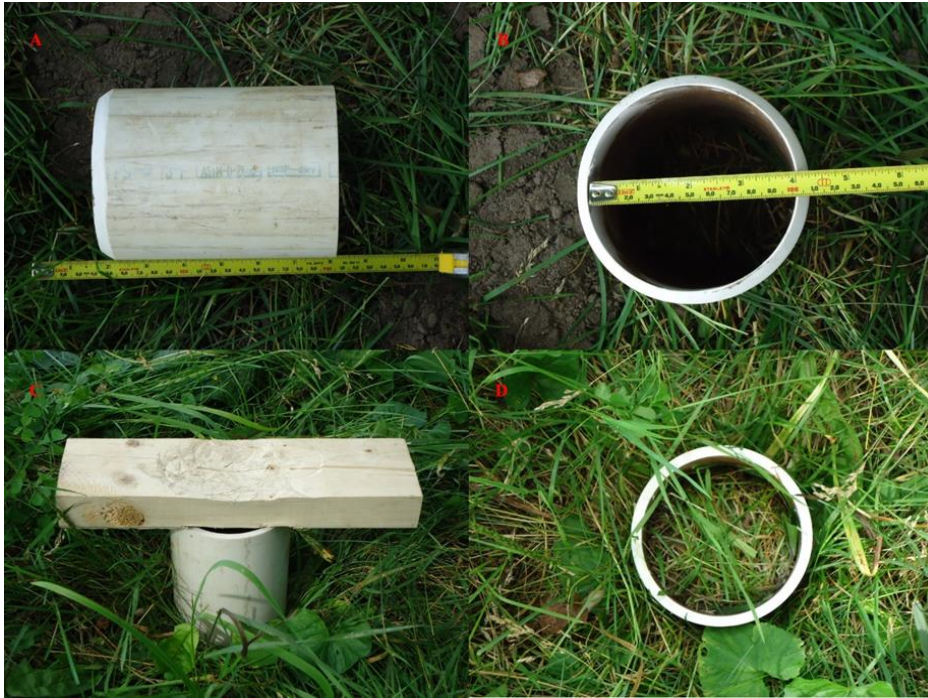
Figure 3-13. Topsoil sample extraction tube dimensions (A and B) and insertion method without disturbing the soil structure or the vegetation (C and D).
