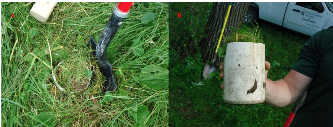
Figure 3-14. (A) Topsoil sample extraction process and (B) topsoil sample extraction without any soil structure or vegetation disturbance.
