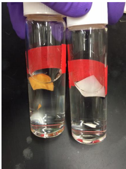
Figure 3.5. Representative images of Fh3 (at left) and Fh3-CTAB3 (at right) composites after digestion in 5 M \text{H}_2\text{SO}_4 for 24 h with constant mixing (0.125 g/L composite loading), indicating greater total solution phase availability of the iron oxide in ternary composites.
