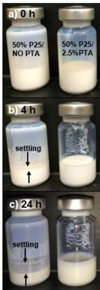
Figure 4-7. Electrospinning sol gels containing 50 wt.% P25 (relative to PAN that would be added) in DMF without PTA (left) and with 2.5 wt.% PTA (relative to final sol gel mass) after (a) initial preparation and 5 h of sonication (0 h), (b) 4 h, and (c) 24 h. P25 began to settle out, as indicated with arrows, after (b) 4 h and (c) 24 h without PTA present.
