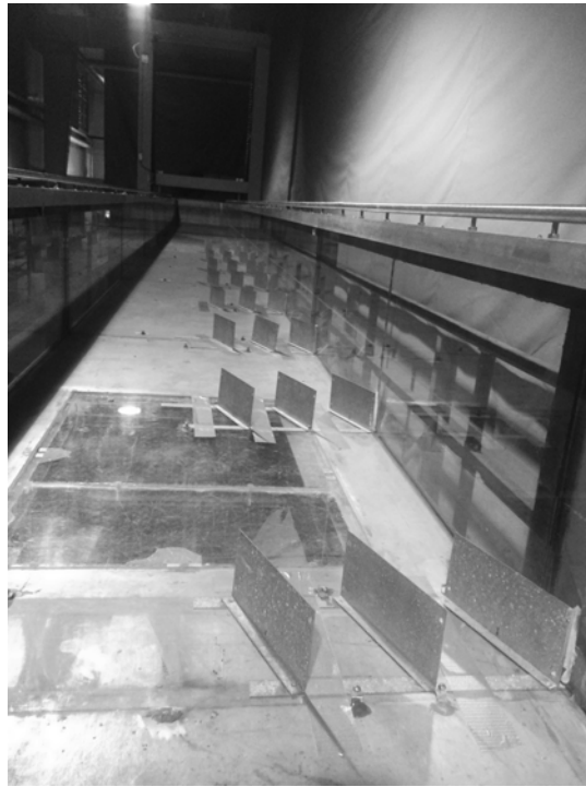
Figure A-11. Vane – wall system used in backwater effect study, angled at 20-degrees. Also known as the vane spur combination. Note: Picture taken from downstream looking upstream.
