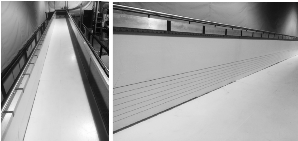
Figure A-4. Flume sheeted covering and lining system utilized in vertical mass transport dye tracer investigations.
