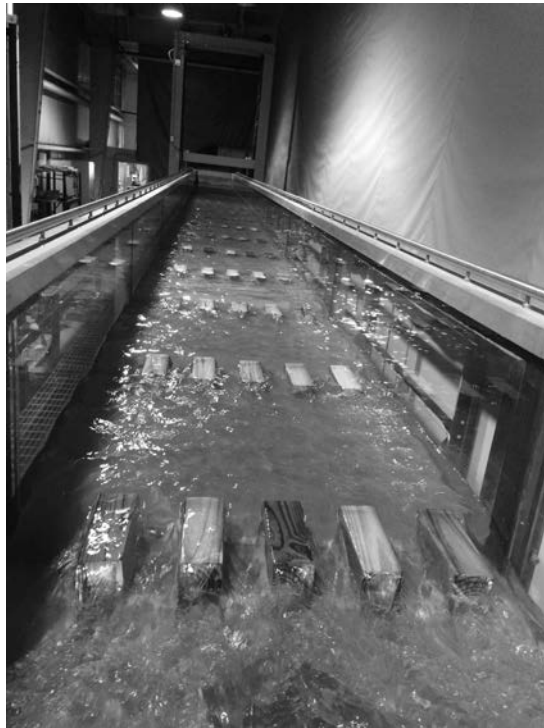
Figure A-16. Metal vane and equivalent full block and frontal projections used in backwater effect study.
