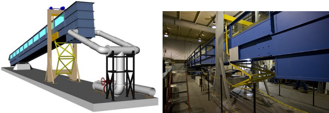
Figure A-1. IIHR’s Tilted flume, a three-foot-wide rectangular flume with length of 54 feet.
