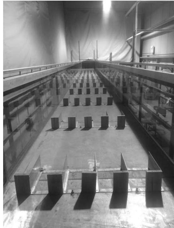
Figure A-16. Metal vane and equivalent full block and frontal projections used in backwater effect study.
