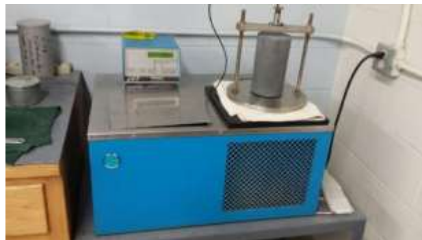
Figure 3-14 Coefficient of Thermal Expansion Testing Apparatus
