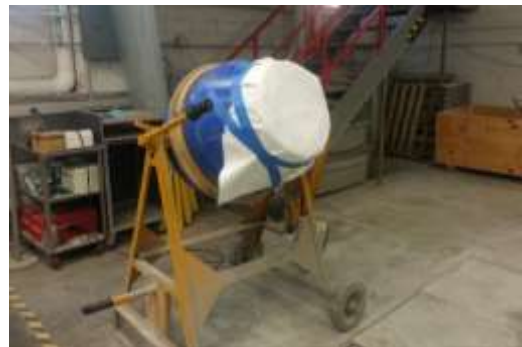
Figure 3-16 2-Cubic Foot Rotational Concrete Mixer covered with paper towels
