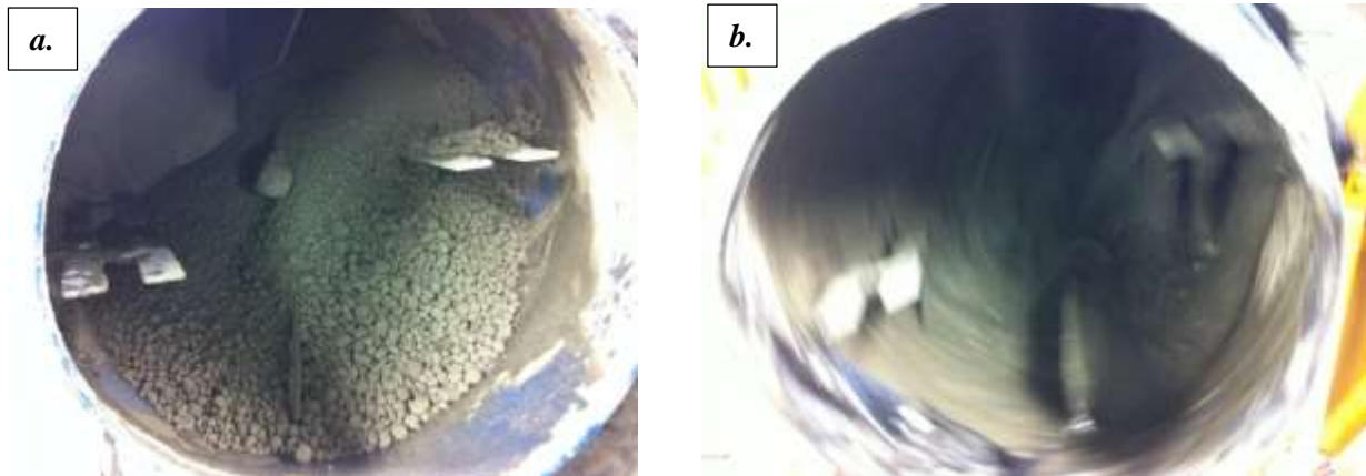
Figure 3-11 Mix 2 Condition after Liquid Additives a) Poor, b) Good
