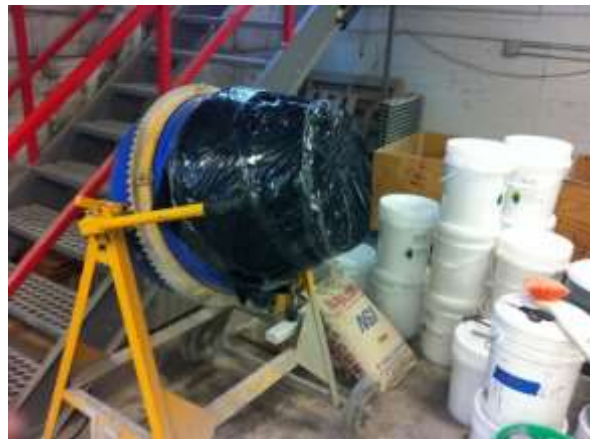
Figure 3-1 2ft 3 Rotational Concrete Drum Mixer Covered with Plastic Bag
