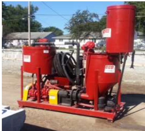
Figure 5-21 Grout Mixer Manufactured by DSI
