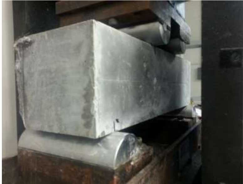
Figure 5-9 Four Point Bending Test on K-UHPC Beam Sample
