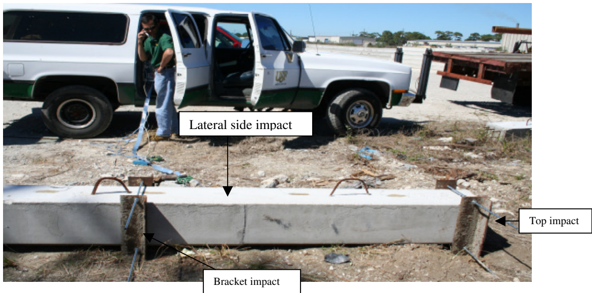
Figure 3.6: Strain Gage Positions 12”x 12”x 40’ Piling
