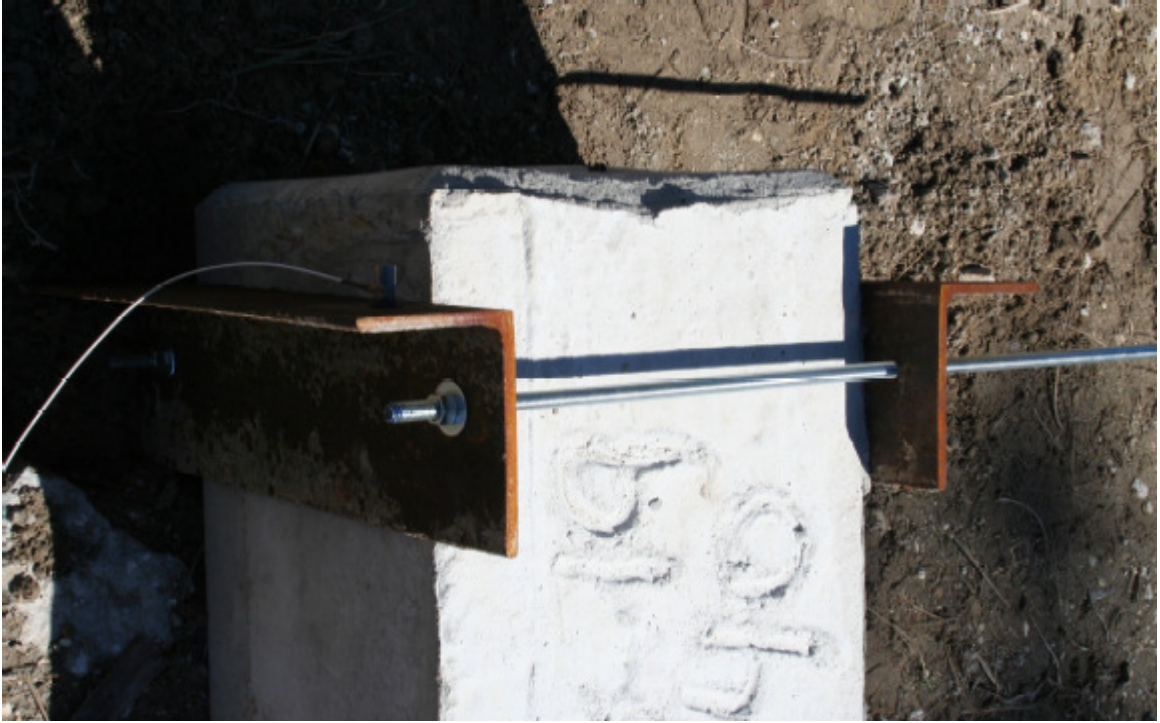
Figure 3.7: Piezoelectric Accelerometer SN45519 Mounted to Bracket
