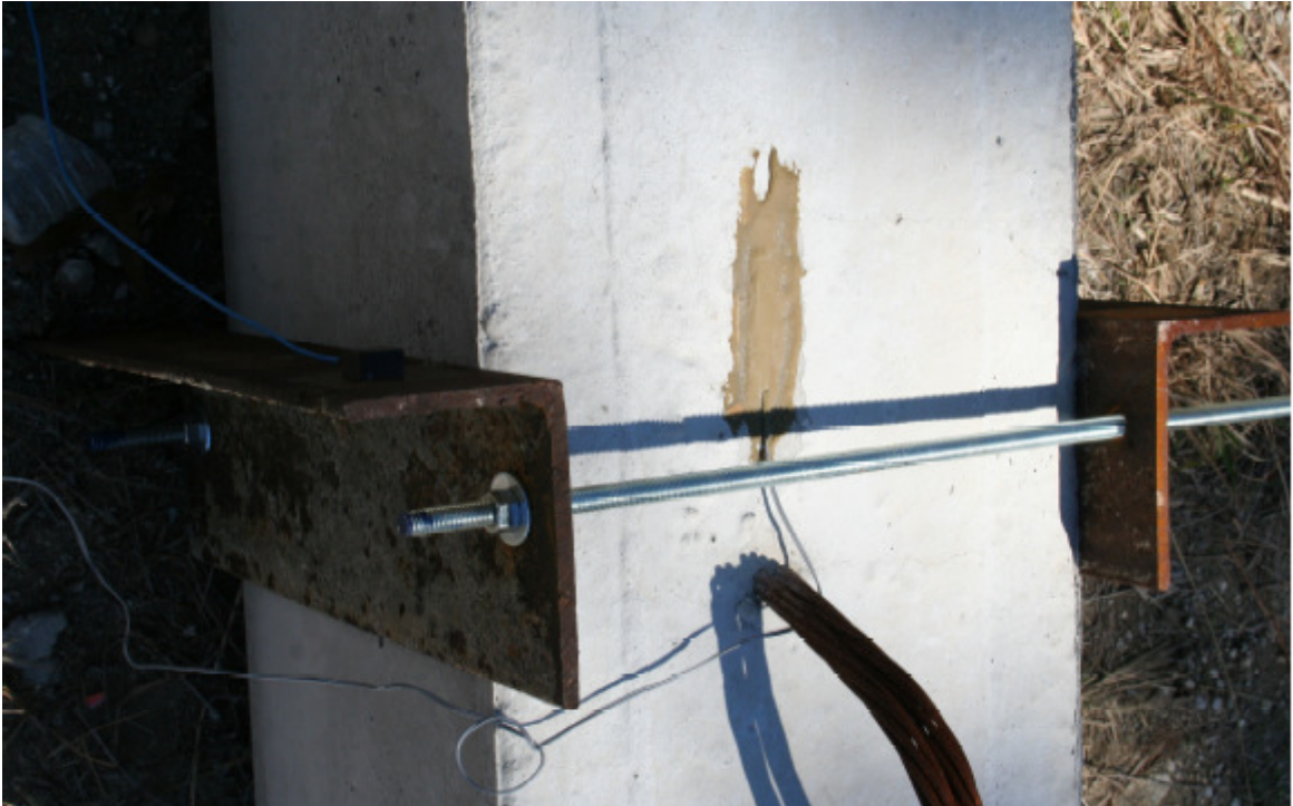
Figure 3.8: Capacitive Accelerometer Mounted to Bracket
