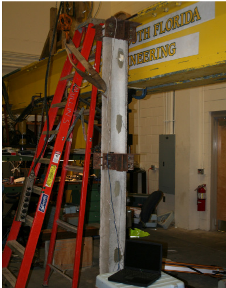
Figure 3.1: Concrete Piling in Lab 6"x 6"x 9'
