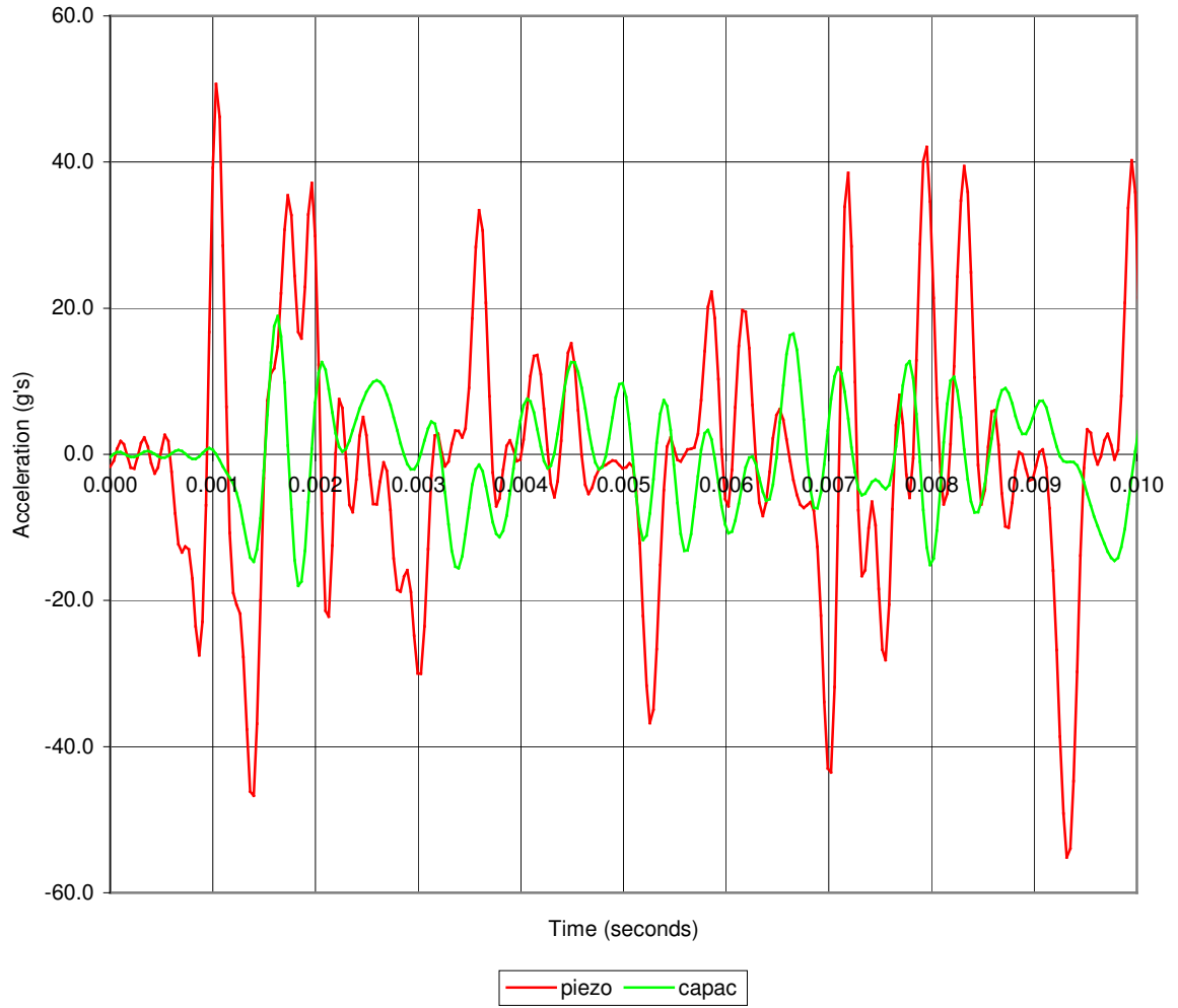
Figure B.2: Top of Piling Impact Accelerations - Test 2
