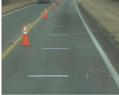
Figure 32: Measurement points marked on the pavement by reflective tapes.
