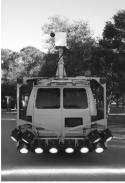
Figure 8: Pavement lighting system and camera.
