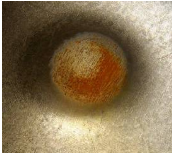
Figure 4-5. Severe Corrosion at a 1-in Convex Dimple Exposed to Solution C. (Picture shows immersed sample surface at 19 days exposure).
