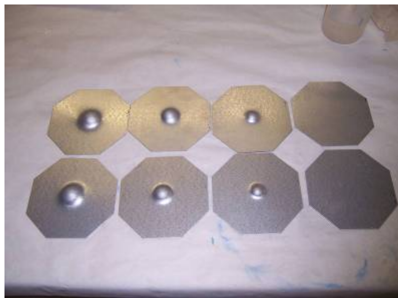
Figure 3-3. Duplicate Aluminized Steel Specimens (Left to Right) 1-in, \frac{3}{4} -in, 9/16-in, and Flat
