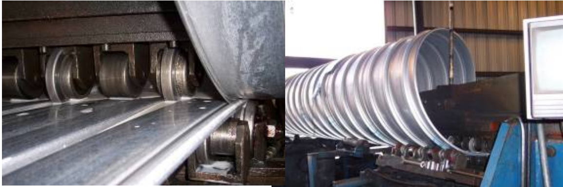
Figure 1-2. Spiral Rib Pipe Manufacturing Process (Dies Used to Form Rib (Left), Forming Spiral Pipe (Right)). [Photograph by the Author]
