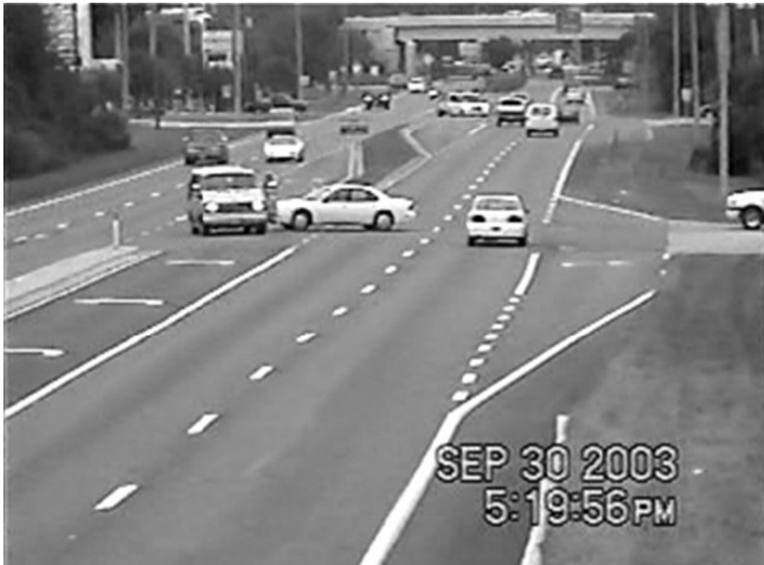
Figure 4.2 Identification of Traffic Conflicts by Swerving
