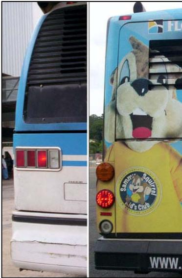
**Figure 1 Vertical and Horizontal Light Configurations**
