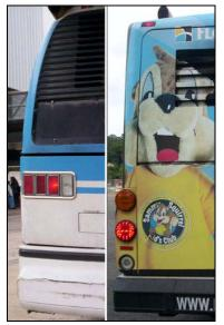
**Figure 1 Vertical and Horizontal Light Configurations**
