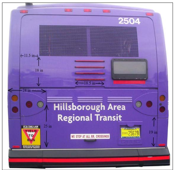
Figure 52 HART Bus with YTB Decal and Dimensions
