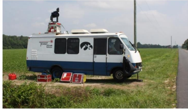
Figure 2. Left: The lidar works by emitting a pulse of light into the atmosphere, collecting backscattered light with a telescope, and ranging using the speed of light. Right: The University of Iowa elastic lidar was set up on a mobile research platform.
