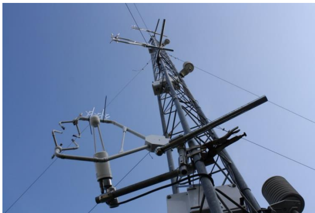
Figure 4. Meteorological tower, with sonic anemometer and IRGA (left) and temperature & humidity probe (bottom right).
