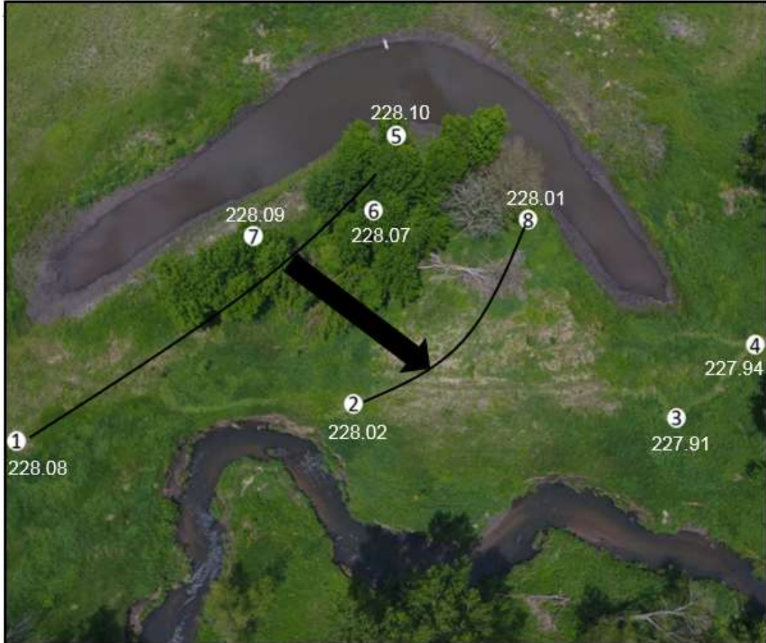
Figure 4.11. Groundwater flow direction estimated on September 12 th , 2016 which flowed in a southeastern direction towards Morgan Creek.
