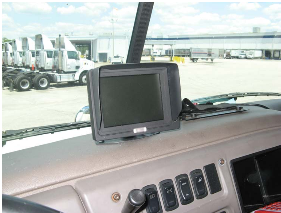
Figure 2.4: LCD 5 inch display mounted on dashboard of large truck.
