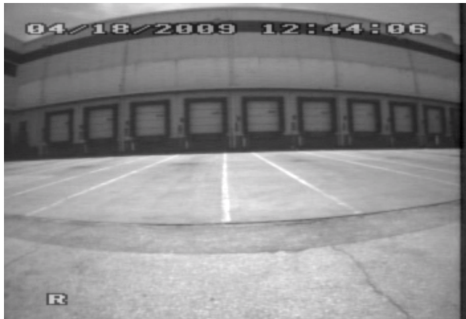
Figure 2.2: View from rearview camera located at 3 ft from ground level.
