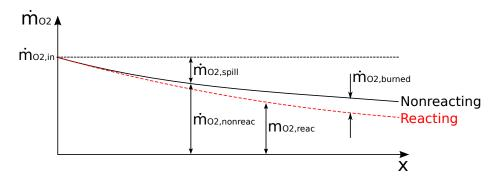
**Figure 86:** Notional oxygen mass flow rates as a function of distance along sampling region with spilled and burned quantities indicated.
