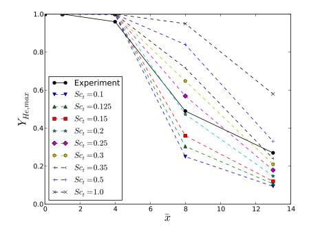
**Figure 25:** Comparisons of maximum helium mass fraction as a function of normalized distance from the injector exit between experiment and numerical simulations at various turbulent Schmidt numbers. Lines are for visual aid only and do not imply a curve shape.
