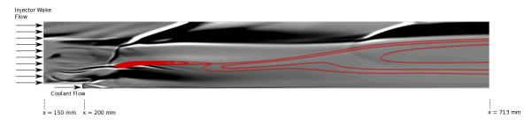
**Figure 99:** Numerical shadowgraphs overlaid with water contours  $Y_{H_2O} = 0.01, 0.02, ..., 0.22$  for tangential film cooling with hydrogen. Coolant temperature of 100 K and B = 20%.
