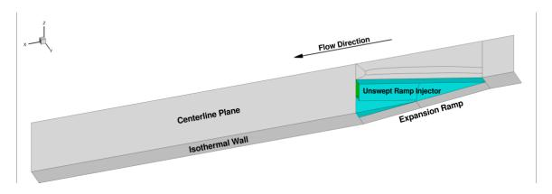
**Figure 38:** The unswept ramp (blue) injector is shown positioned in the portion of the computational domain where performance sampling occurs.
