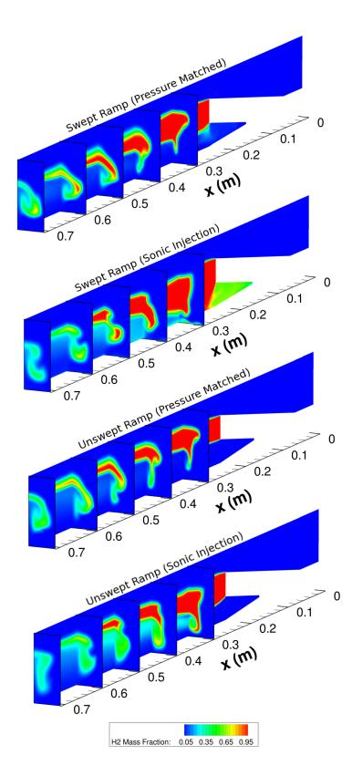
**Figure 57:** Fence plots of hydrogen mass fraction for the ramp injection cases without the base expansion wedge.
