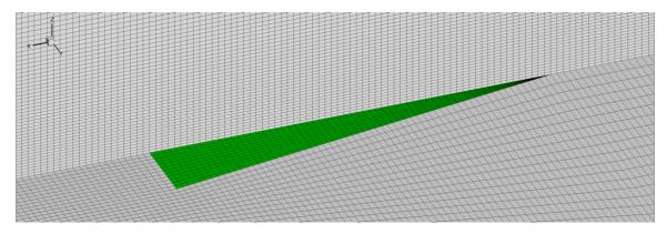
**Figure 41:** The computational grid in the vicinity of the wedge injector (green) is shown.
