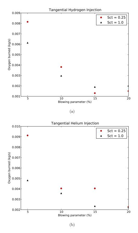
**Figure 109:** Changes in mass flow of oxygen burned for tangential, secondary hydrogen and helium injection is shown.
