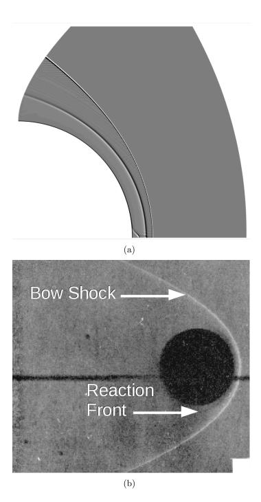
**Figure 75:** (a) Numerical shadowgraph of a Mach 5, 20 mm spherically blunted projectile fired into 0.1 atm quiescent H2-Air is shown and compared to the (b) experimental shadowgraph [96].
