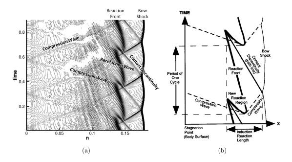
**Figure 136:** Contour lines of (a) density on the stagnation streamline as a function of time for Ruegg and Dorsey experiment Case 2 and (b) 1D mechanism for the regular, unsteady regime by Matsuo (reproduced with permission).
