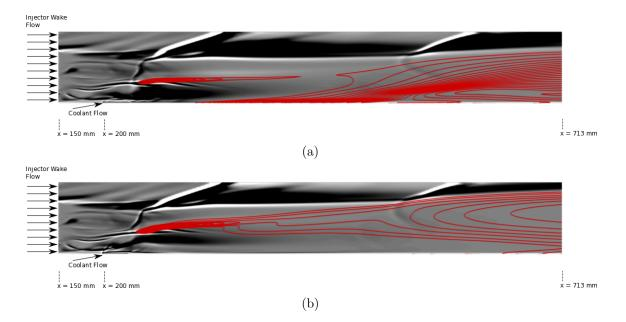
**Figure 104:** Numerical shadowgraphs overlaid with water contours  $Y_{H_2O} = 0.01$ , 0.02, ..., 0.22 for 10 degree film cooling with helium. B = 15% and ambient coolant temperatures of (a) 100 K and (b) 740 K are shown.
