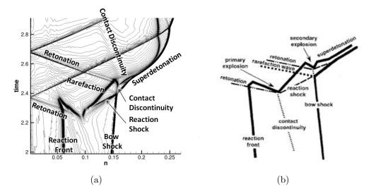
**Figure 138:** A detail view of the (a) stagnation streamline density contours from the present simulation (Case 3) compared to a (b) 1D sub-mechanism of the large-disturbance regime as proposed by Matsuo and Fujii [97] (reproduced with permission).
