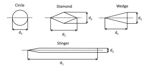
Figure 30: Notional geometry for flush wall injectors.
