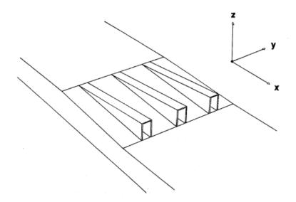
Figure 21: A schematic of the Waitz expansion ramp injector is shown (from [62]).
