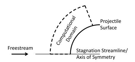
Figure 124: Schematic of the current state of the art for solving flow ahead of a blunted projectile.
