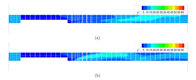
**Figure 54:** Contour plots of wall  $y^+$  for the full flowpath of the unswept ramp fuel injector with expansion wedge at both a (a) pressure matched and (b) sonic pressure condition. Flow is from the left to the right and the ramp itself is blanked out.
