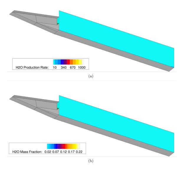
**Figure 91:** Unswept ramp injector contours of (a) water production and (b) water mass fraction in the flow domain of interest. Flow is from the upper left to the lower right.
