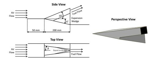
Figure 31: Side-, top-, and perspective-view geometry for modified ramp injectors.
