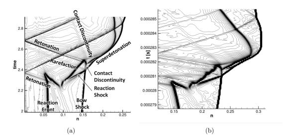
**Figure 134:** A detail view of density contours on the stagnation streamline as a function of time for Case 3 for the (a) QUIVR quasi-1D simulation and (b) high-fidelity, 2D simulation produced using VULCAN. Note that the computed results are non-dimensional in time while the high-fidelity plot is in seconds.
