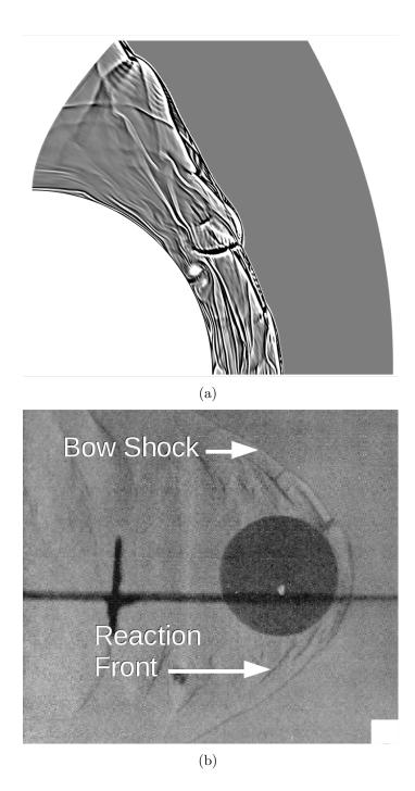
**Figure 77:** (a) Numerical shadowgraph solution of a Mach 4.8, 20 mm spherically blunted projectile fired into 0.5 atm quiescent H2-Air is shown and compared to the (b) experimental shadowgraph [96].
