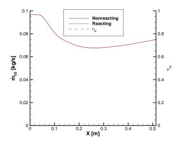
**Figure 92:** Mass flow rates of oxygen and combustion efficiency downstream of strut without autoignition mitigation.
