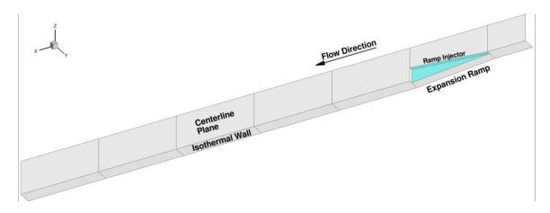
Figure 23: The expansion ramp geometry of Waitz for the validation study is shown.
