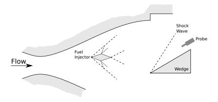
**Figure 8:** A reproduced schematic of the PMSIC experiment conducted by by Rubins and Rhodes [8] is shown.
