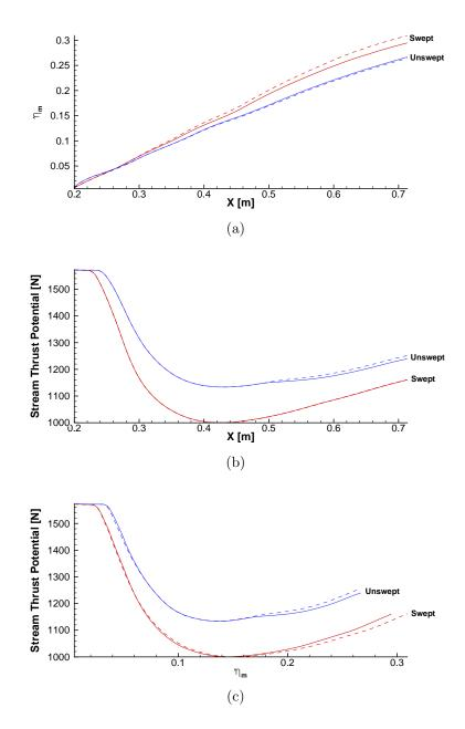
**Figure 60:** Performance of ramp injection concepts for sonic pressure: (a) mixing efficiency versus x, (b) stream thrust potential versus x, and (c) stream thrust potential versus mixing efficiency. Dashed lines indicate cases with the expansion wedge feature.
