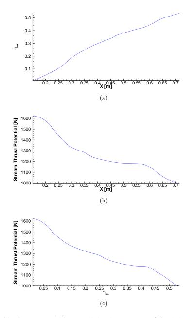
**Figure 64:** Performance of the strut injection concept: (a) mixing efficiency versus x, (b) stream thrust potential versus x, and (c) stream thrust potential versus mixing efficiency.
