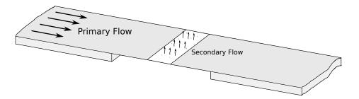
Figure 68: Notional diagram of wall transpiration.
