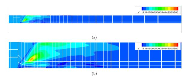
**Figure 48:** Contour plots of wall  $y^+$  for the (a) full flowpath and (b) in the vicinity of the diamond fuel injector. Flow is from the left to the right and hydrogen issues from the injector out of the page.
