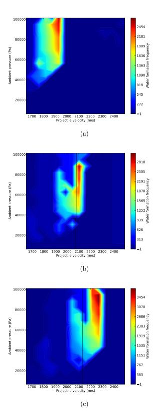
**Figure 139:** Filled contours of reaction front frequency as a function of projectile velocity and ambient pressure for (a) lean, (b) stoichiometric, and (c) rich equivalence ratios. The black line on the latter two plots indicate the Chapman-Jouget detonation velocity.
