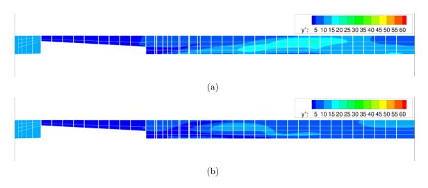
**Figure 56:** Contour plots of wall  $y^+$  for the full flowpath of the swept ramp fuel injector with expansion wedge at both a (a) pressure matched and (b) sonic pressure condition. Flow is from the left to the right and the ramp itself is blanked out.
