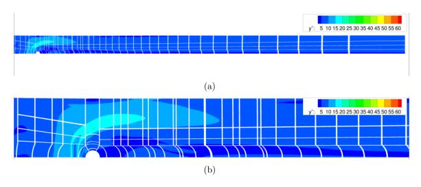
**Figure 46:** Contour plots of wall  $y^+$  for the (a) full flowpath and (b) in the vicinity of the fuel injector. Flow is from the left to the right and hydrogen issues from the injector out of the page.
