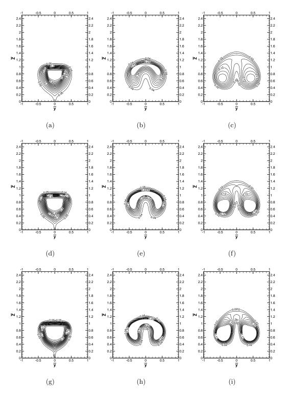
**Figure 27:** Numerically solved contours for helium mass fraction are shown for (a) - (c)  $Sc_t = 0.25$ , (d) - (f)  $Sc_t = 0.5$ , and (g) - (i)  $Sc_t = 1.0$ . The columns sequentially show normalized x coordinates of 4, 8, and 13 from the injector exit.
