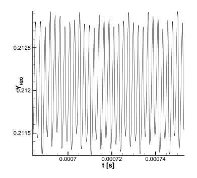
**Figure 83:** Water mass fraction as a function of time at the projectile wall for the Mach 4.47 case.
