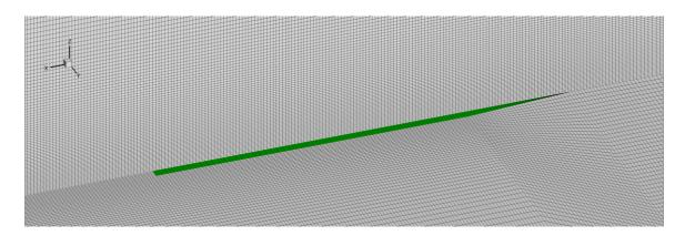
**Figure 43:** The computational grid in the vicinity of the stinger injector (green) is shown.
