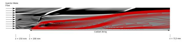
**Figure 106:** Numerical shadowgraphs overlaid with water contours  $Y_{H_2O} = 0.01$ , 0.02, ..., 0.22 for transpiration cooling with helium. Parameters B = 20% and W = 25% are shown.
