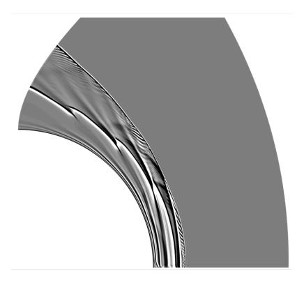
**Figure 81:** Numerical shadowgraph for the Mach 4.47 projectile case with stoichiometric H2-air at 0.421 atm and 292 K ambient conditions.
