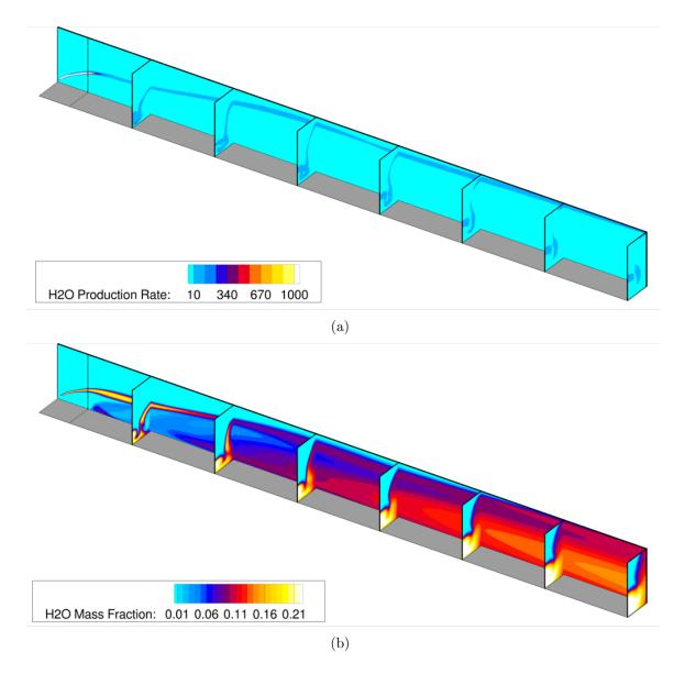
**Figure 87:** Stinger injector contours of (a) water production and (b) water mass fraction in the flow domain of interest. Flow is from the upper left to the lower right.
