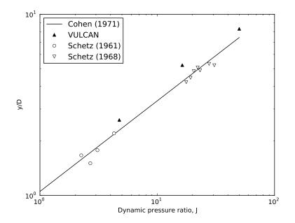
**Figure 20:** Vertical displacement of the Mach disk midpoint as a function of dynamic pressure.
