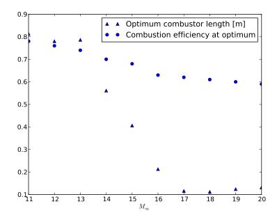
**Figure 118:** Optimum combustor length and combustion efficiency at that point at different trajectory points.
