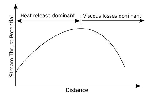
Figure 115: A notional trend of thrust potential versus distance in a combustor.
