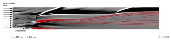
**Figure 100:** Numerical shadowgraphs overlaid with water contours  $Y_{H_2O} = 0.01$ , 0.02, ..., 0.22 for tangential film cooling with hydrogen. The coolant temperature is 740 K and B = 20%.
