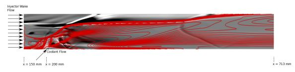
**Figure 102:** Numerical shadowgraphs overlaid with water contours  $Y_{H_2O} = 0.01$ , 0.02, ..., 0.22 for 45 degree film cooling with hydrogen. The coolant temperature is 740 K and B = 20%.
