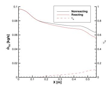
**Figure 90:** Mass flow rates of oxygen and combustion efficiency downstream of strut without autoignition mitigation.
