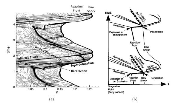
**Figure 137:** Contour lines of (a) density on the stagnation streamline as a function of time for Ruegg and Dorsey experiment Case 3 and (b) 1D mechanism for the regular, unsteady regime by Matsuo and Fujii (reproduced with permission).
