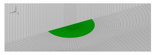
**Figure 40:** The computational grid in the vicinity of the circular injector (green) is shown.
