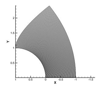
**Figure 74:** The grid used in the validation study is shown with every tenth grid point normal to the surface and every third grid point tangential to surface.
