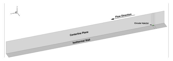
**Figure 34:** The circular injector (green) is shown positioned in the portion of the computational domain where performance sampling occurs.
