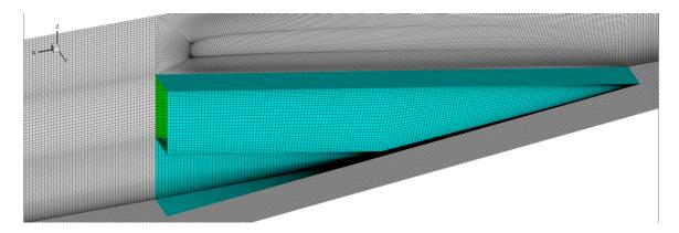
**Figure 44:** The computational grid in the vicinity of the unswept ramp wedge injector (blue) is shown.
