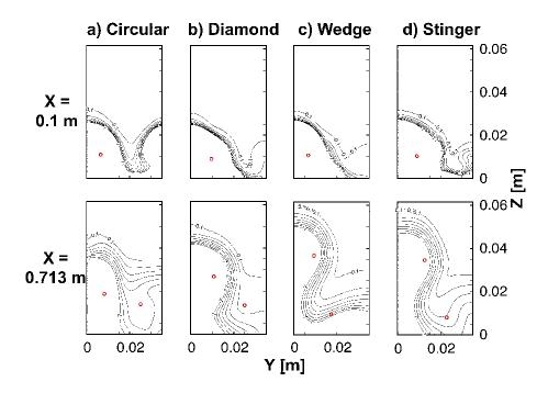
**Figure 52:** Fuel equivalence ratio contours for the (a) circular, (b) diamond, (c) wedge, and (d) stinger injection case at x = 0.1 m and 0.713 m. Lines are plotted as  $\phi = 0.1, 1, 2...7$ . Circular marker indicates vortex center.
