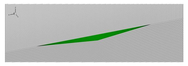
**Figure 42:** The computational grid in the vicinity of the diamond injector (green) is shown.
