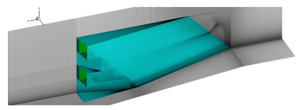
**Figure 45:** The computational grid in the vicinity of the strut injector (blue) is shown.
