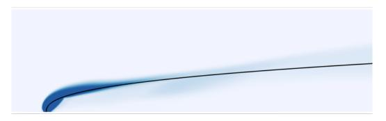
**Figure 18:** The centerline hydrogen mass fraction field of a converged VULCAN case where J = 4.75 is shown compared to the analytical relation from Equation 3 with m = 1, n = 2.55.
