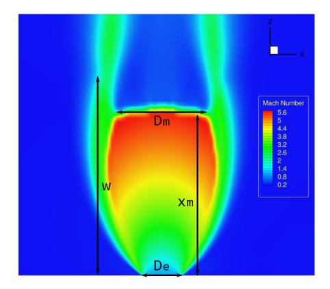
**Figure 14:** A plane bisecting the sonic jet is shown from the converged case of jet pressure ratio equal to 20. Parameters of the jet are shown, consisting of wavelength, w, Mach disk diameter,  $D_m$ , exit diameter,  $D_e$ , and Mach disk standoff distance  $x_m$ .
