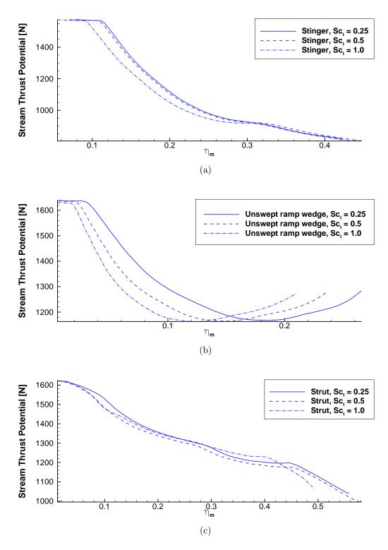
**Figure 67:** Comparisons of stream thrust potential versus mixing efficiency between the (a) stinger, (b) unswept ramp with wedge, and (c) strut injectors for  $Sc_t = 0.25 - 1.0$ .
