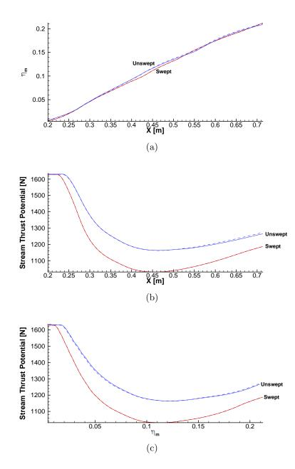
**Figure 58:** Performance of ramp injection concepts for matched pressure: (a) mixing efficiency versus x, (b) stream thrust potential versus x, and (c) stream thrust potential versus mixing efficiency. Dashed lines indicate cases with the expansion wedge feature.
