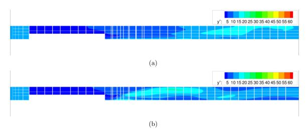
**Figure 53:** Contour plots of wall  $y^+$  for the full flowpath of the unswept ramp fuel injector with cavity at both a (a) pressure matched and (b) sonic pressure condition. Flow is from the left to the right and the ramp itself is blanked out.
