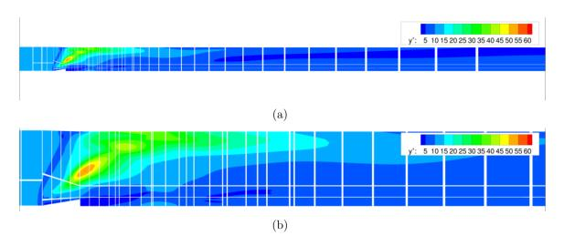
**Figure 49:** Contour plots of wall  $y^+$  for the (a) full flowpath and (b) in the vicinity of the diamond fuel injector. Flow is from the left to the right and hydrogen issues from the injector out of the page.
