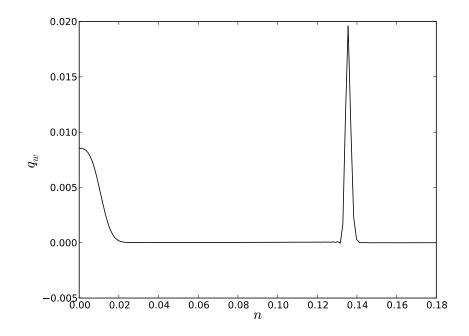
**Figure 128:** The solution of nondimensional heat flux as a function of distance from the wall is shown for a 63.5 mm projectile with  $T_w = 3000$  K and traveling at  $M_{\infty} = 5.72$  at an altitude of 35 km.
