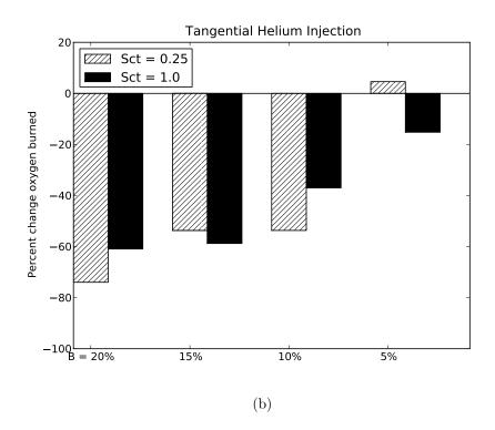
**Figure 110:** Percent changes in mass flow of oxygen burned for tangential, secondary hydrogen and helium injection is shown.
