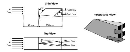
Figure 32: Side- and top-view geometry for strut injector.
