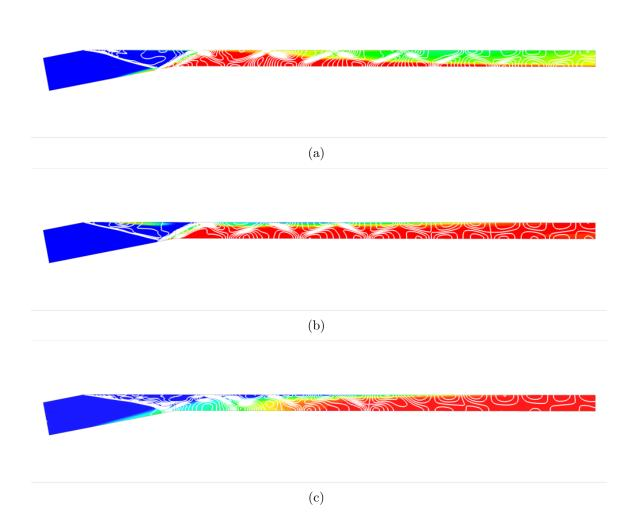
**Figure 119:** Filled contours of water mass fraction superimposed with lines of constant pressure for the Mach 12 strut flowfield at y = (a) 0, (b) 0.0172, and (c) 0.0345 m
