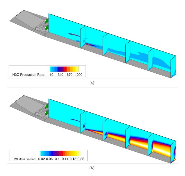
**Figure 89:** Strut injector contours of (a) water production and (b) water mass fraction in the flow domain of interest. Flow is from the upper left to the lower right.
