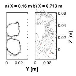
**Figure 65:** Fuel equivalence ratio contours for the strut injector case at x = 0.16 and 0.713 m m. Lines are plotted as  $\phi = 0.1, 1, 2...7$ . Circular marker indicates vortex center.
