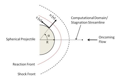
Figure 126: The flow schematic and coordinate system for the quasi-1D equations are shown.
