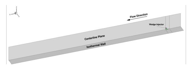
**Figure 35:** The wedge injector (green) is shown positioned in the portion of the computational domain where performance sampling occurs.
