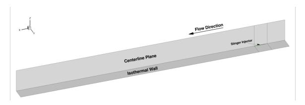
**Figure 37:** The stinger injector (green) is shown positioned in the portion of the computational domain where performance sampling occurs.
