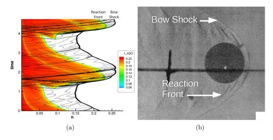
**Figure 133:** (a) Contours of water mass fraction on the stagnation streamline overlaid with contour lines of pressure as a function of non-dimensional time for Ruegg and Dorsey experiment Case 3. (b) An annotated experimental shadowgraph captured by Ruegg and Dorsey for the same conditions is shown for comparison.
