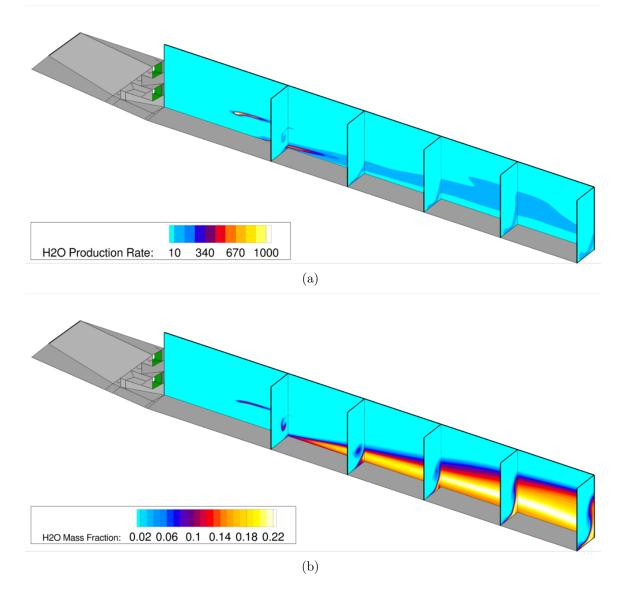
**Figure 111:** Strut injector contours of (a) water production and (b) water mass fraction in the flow domain of interest using the Ó Conaire mechanism without hydrogen peroxide. Flow is from the upper left to the lower right.
