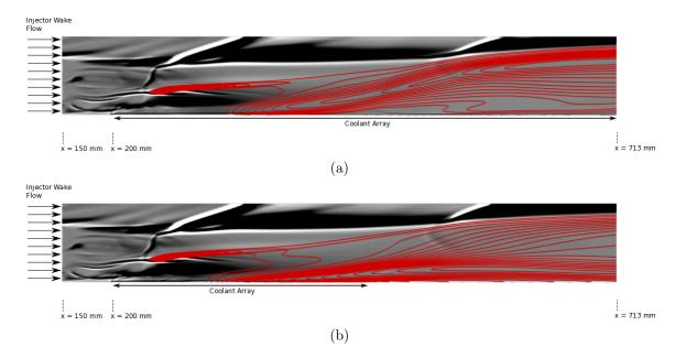
**Figure 108:** Numerical shadowgraphs overlaid with water contours  $Y_{H_2O} = 0.01$ , 0.02, ..., 0.22 for transpiration cooling with helium. B = 20% and patch sizings of (a) W = 25% and (b) L = 50% are shown.
