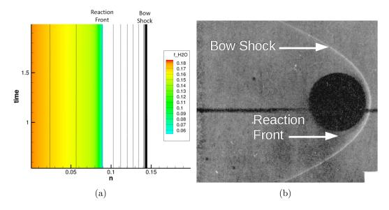
**Figure 131:** (a) Contours of water mass fraction on the stagnation streamline overlaid with contour lines of pressure as a function of non-dimensional time for Ruegg and Dorsey experiment Case 1. (b) An annotated experimental shadowgraph captured by Ruegg and Dorsey for the same conditions is shown for comparison.
