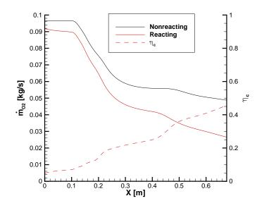
**Figure 88:** Mass flow rates of oxygen and combustion efficiency downstream of stinger without autoignition mitigation.
