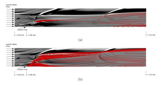
**Figure 101:** Numerical shadowgraphs overlaid with water contours  $Y_{H_2O} = 0.01, 0.02, ..., 0.22$  for 10 degree film cooling with hydrogen. B = 20% and ambient temperatures of (a) 100 K and (b) 740 K are shown.
