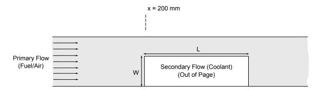
Figure 95: Schematic diagram of wall transpiration.
