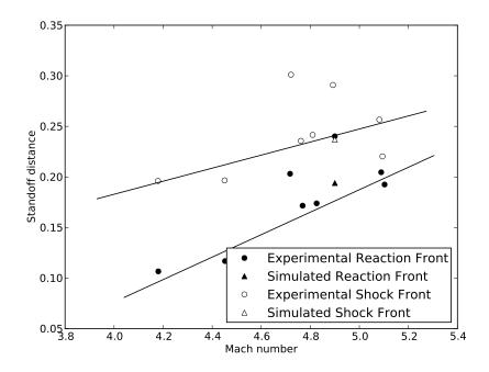
**Figure 79:** A comparison is shown between shock and reaction front standoff distances for experiment and the present simulation at 0.25 atm.
