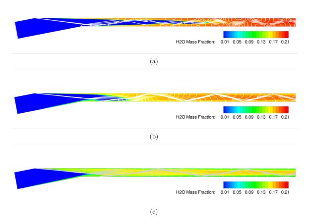
**Figure 116:** Contours of water mass fraction overlaid with lines of constant pressure for Mach numbers (a) 11, (b) 15, and (c) 20.
