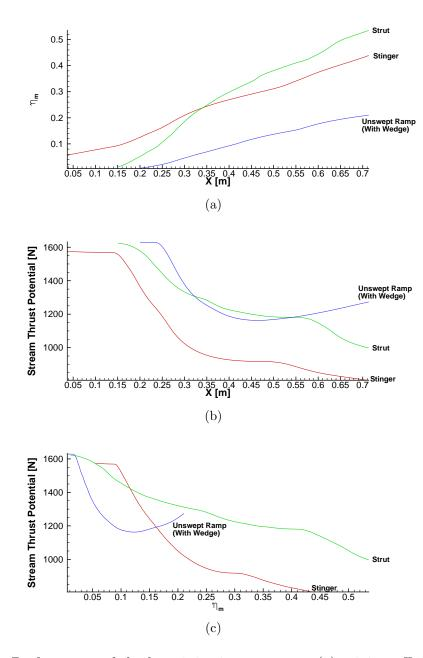
**Figure 66:** Performance of the best injection concepts: (a) mixing efficiency versus x, (b) stream thrust potential versus x, and (c) stream thrust potential versus mixing efficiency.
