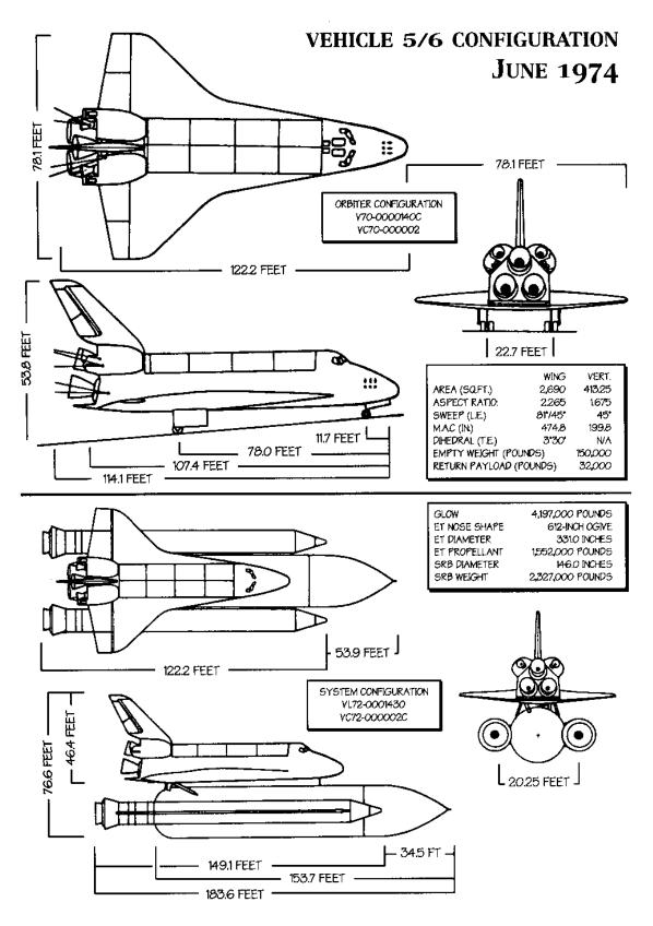
Figure 70: The Final Space Shuttle Orbiter Configuration [61]
