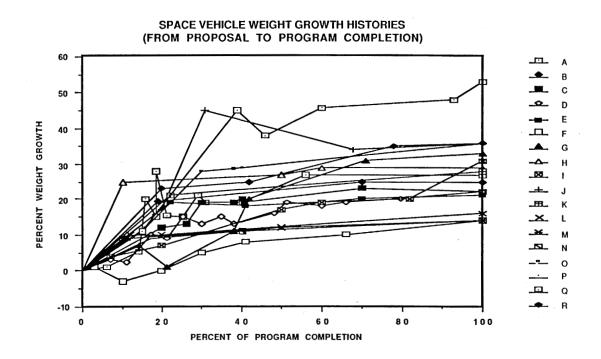
Figure 3: Dry Mass Growth of Satellites [53]
