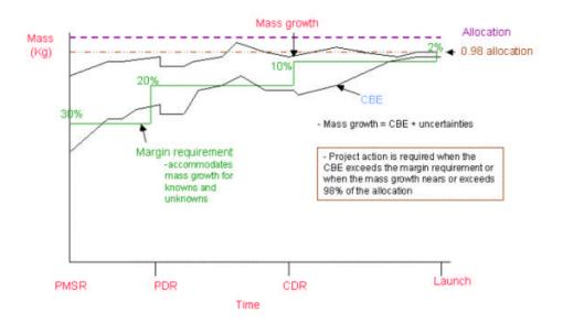
Figure 15: Jet Propulsion Laboratory Mass Growth Standard [150]
