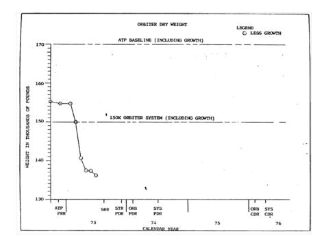
Figure 72: Space Shuttle Mass Changes as of July 1973[95]
