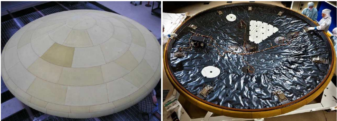
Figure 3: Completed MSL heatshield and underside with MEDLI system installed.
