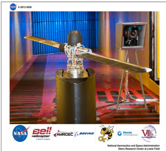
Figure 31: Model Bell 206 tail rotor used in an icing tunnel test at NASA Glenn Research Center's Icing Research Tunnel
