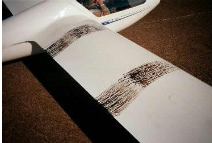
Figure 18: Flow visualization for a straight wing aircraft [41]
