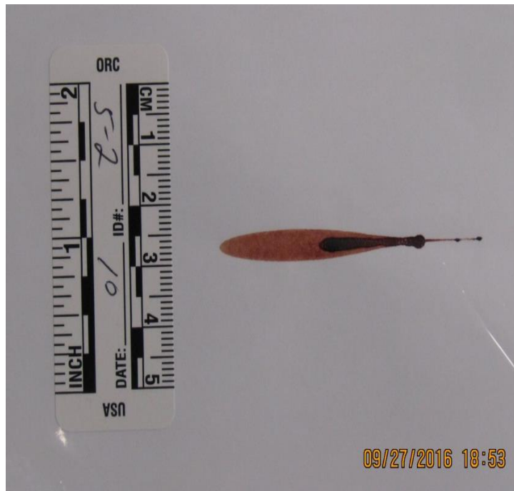
Figure 23. Normal density blood sample dropped at a 10^\circ angle.
