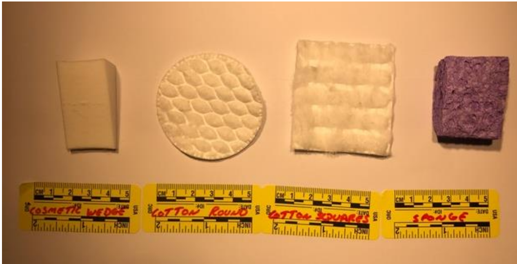
Figure 54. Materials tested to hold blood samples for blood spatter simulations.
