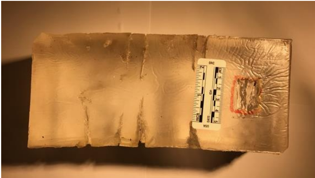
Figure 56. Ballistic gel target with cut out for blood samples.
