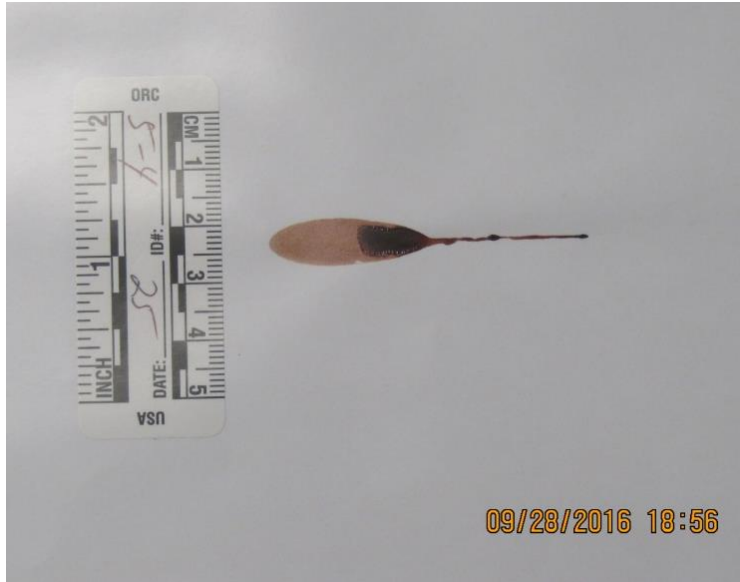
Figure 26. Normal density blood sample dropped at a 25° angle.
