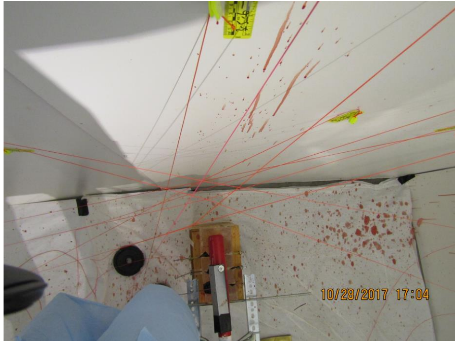
Figure 104. Simulation 3.5 string method construction.
