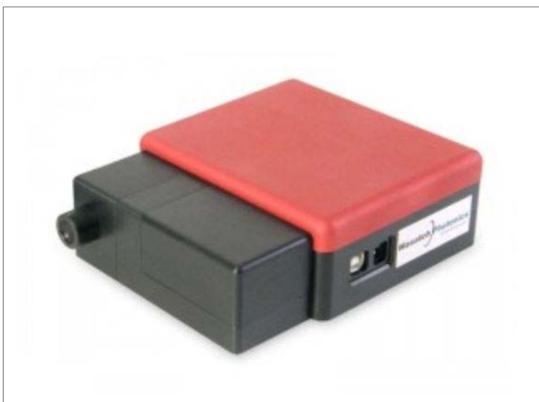
Figure 39. Photograph of Wasatch Raman 785L spectrometer. ( http://wasatchphotonics.com/systems/vph-spectrometers/raman-flourescence/stroker-785l/ )
