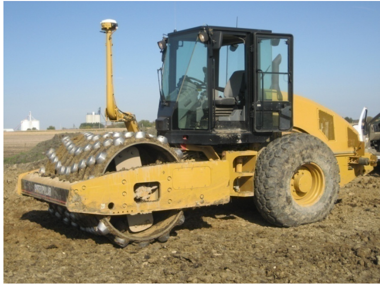
Figure 26: Compactor used for TH60 project (specifications unknown)
