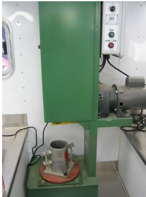
Figure 60: Automated mechanical rammer for impact compaction test
