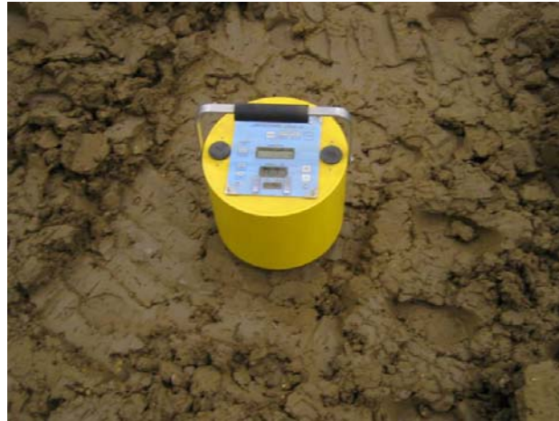
Figure 65: Modulus determination using soil stiffness gauge
