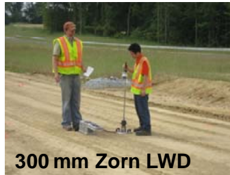
Figure 83: Field conditions and in-situ testing from North Carolina Hwy 311 project
