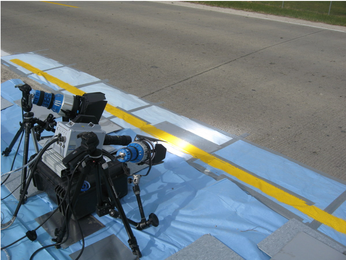
Figure 3.6: High-speed camera setup on side of roadway.
