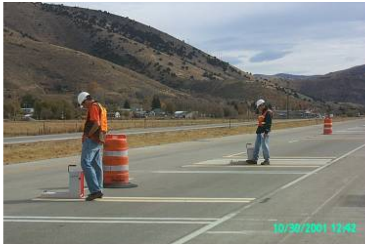
Figure 2.1: Utah's NTPEP Test Deck. Source: Utah T2 Center
