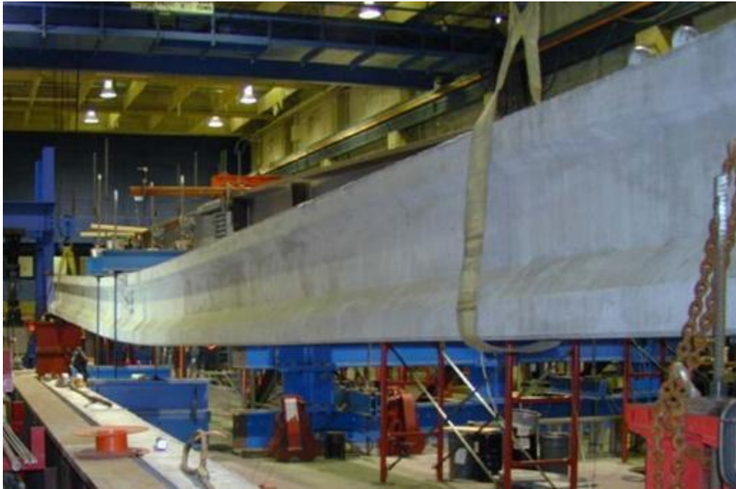
Figure 2.28. An 80-ft (24-m) girder showing a deflection of 17 in. (430 mm) (Graybeal 2005)
