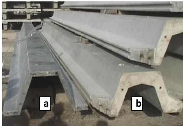
Figure 2.43. Comparison of a) SCFRC and b) conventional concrete sheet piles (Grünewald 2004)
