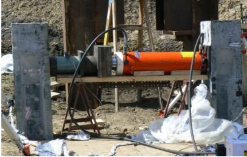
Figure 5.34. View showing the lateral load test set-up at the beginning of the load test
