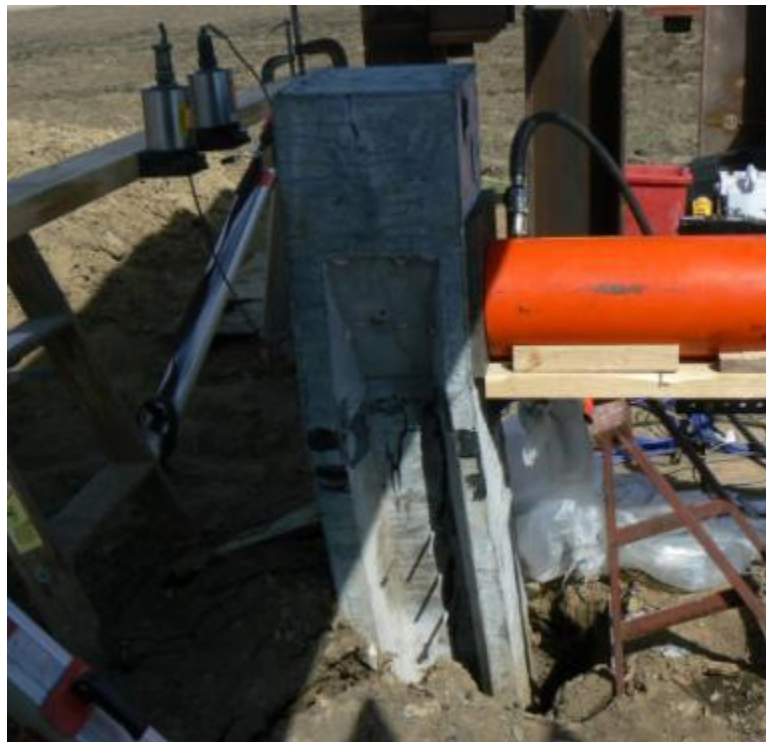
Figure 5.46. Bending of UHPC pile P1 under a lateral displacement of 7.87 in. (200.0 mm) after the shear failure began to occur
