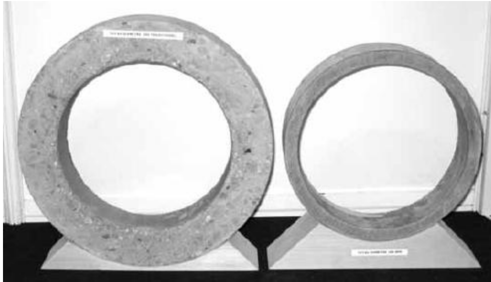
Figure 2.30. Reduction in pipe wall thickness of UHPC (right) compared to an equivalent pipe in normal concrete (left) (Droll 2004)
