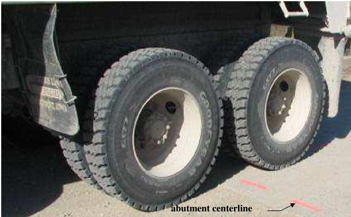
Figure 3.11. BCB Truck Tandem Centroid Centered Over Abutment.
