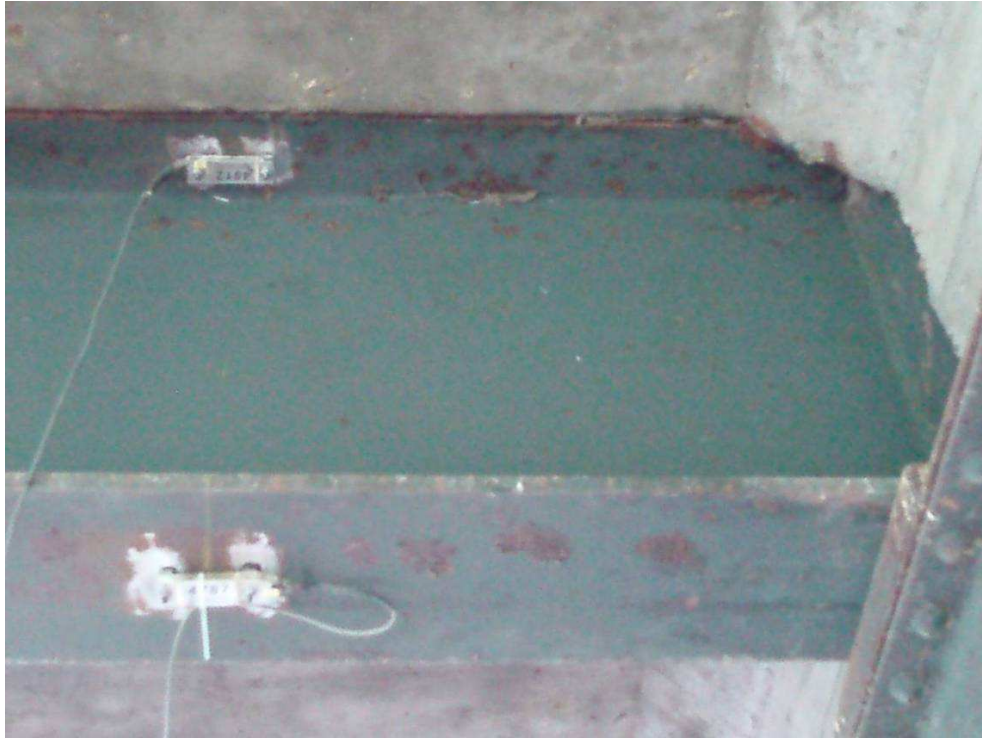
Figure 6.6. CCB Bearing Transducer Locations.
