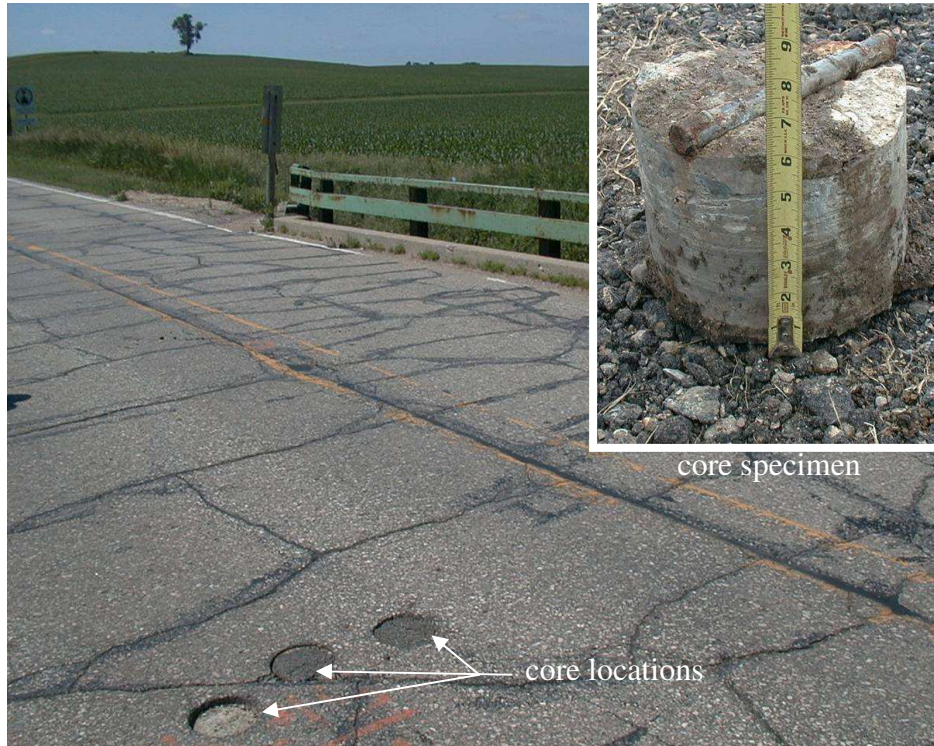
Figure 4.3. MCB Core Locations and Retrieved Core Specimen.
