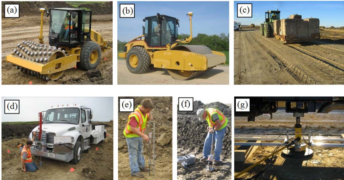
FIG. 4.2— (a) CP-563 roller, (b) CS-563 roller, (c) Towed pneumatic dual-wheel test roller with 650 kPa contact tire pressure, (d) Shelby tube sampler, (e) DCP, (f) Zorn 200-mm diameter plate LWD, (g) 6.2 kN capacity static plate load test setup.
