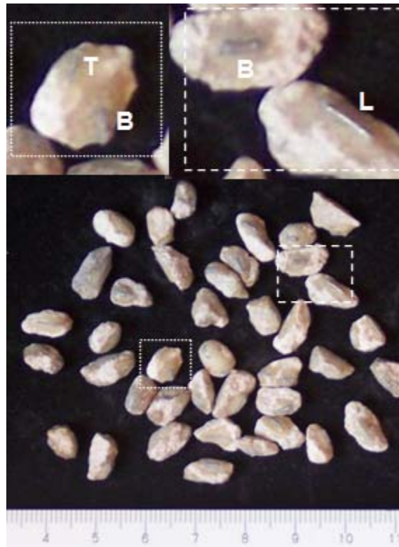
Figure 3.3. Solder marked particles used in analysis with zoom into B, L, and T solder piece examples. Ruler scale is in centimeters.
