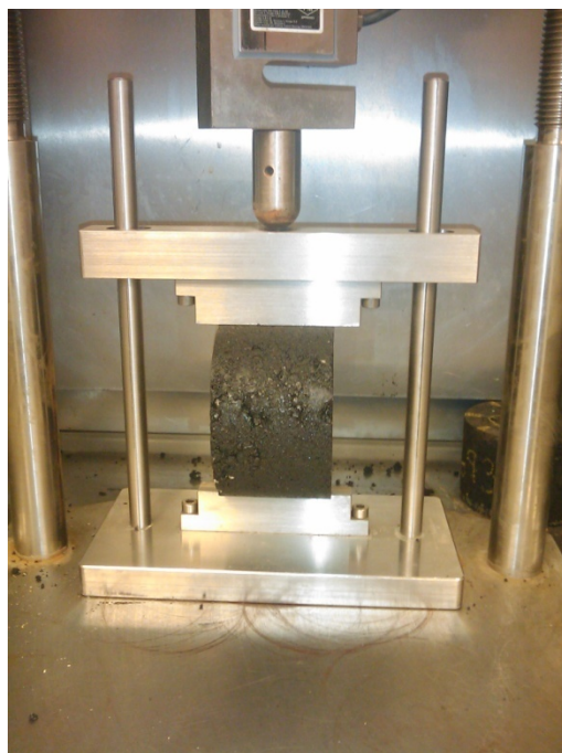
Figure 3-4 Indirect Tensile Strength Test Setup
