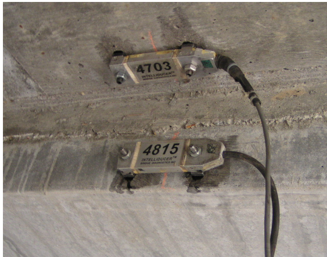
Figure 3.11. BDI strain transducers attached to concrete.
