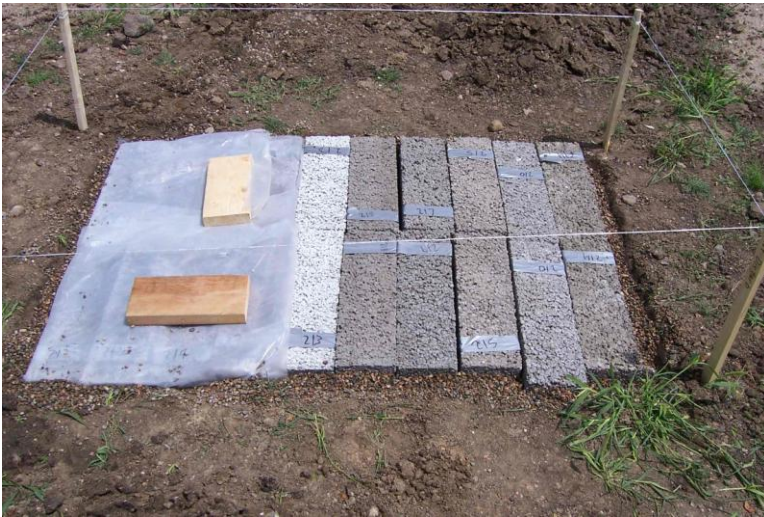
Figure 48. Initial beam curing
