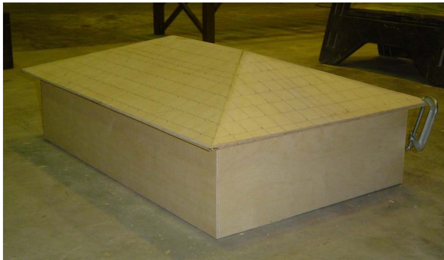
Figure 6.3c. 1/16 – Scale model of the low-rise test building after gluing the walls, eaves, and roof
