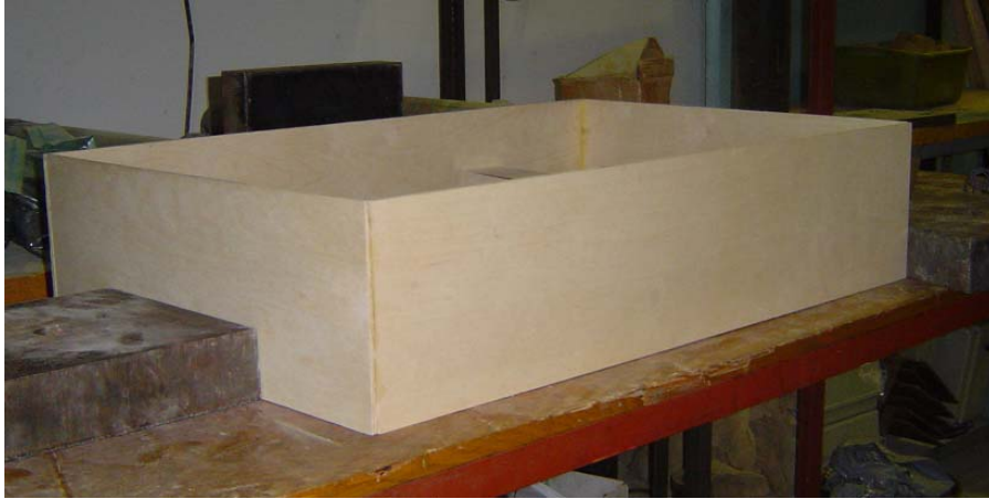
Figure 6.3a. 1/16 – Scale model of the low-rise test building after gluing the walls
