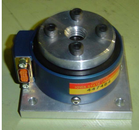
Figure 6.9. JR3 used to measure the wind induced structural forces and moments at the base of the test model
