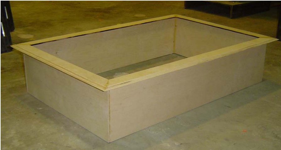
Figure 6.3b. 1/16 – Scale model of the low-rise test building after gluing the walls and eaves
