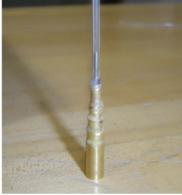
Figure 3.7. Adapter used to connect the 3/16 inch pressure port to the 1/25 inch vinyl tubing
