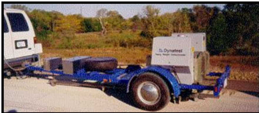
Figure 17: Falling Weight Deflectometer (Cable J. K., et al. 2003)
