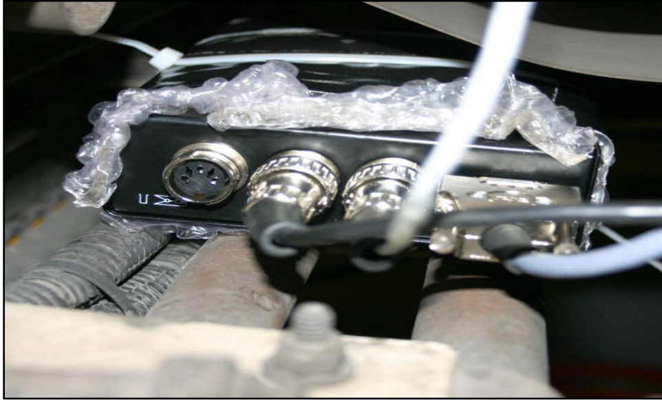
Figure 3.12: Digital data acquisition port
