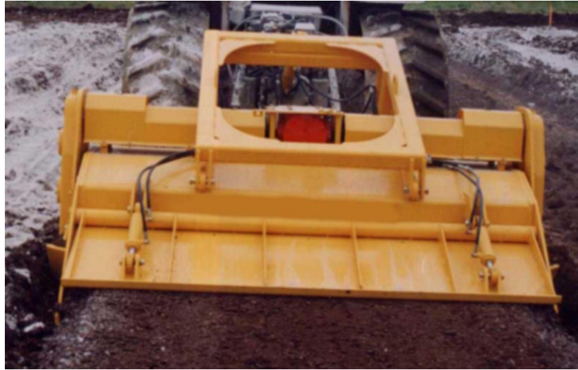
FIGURE 3.1 Type MGM 250 soil mixer (3)
