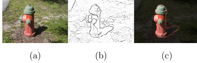
Figure A.2: Example of Problematic Segmentation due to Shadow. (a) test image. (b) edge map by combining Pb and hue gradient. (c) segmentation using edge map in (b).
