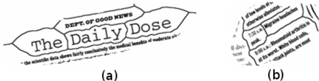
Figure 3.8: Text-line direction can help merging the over-segmented regions as shown above.
