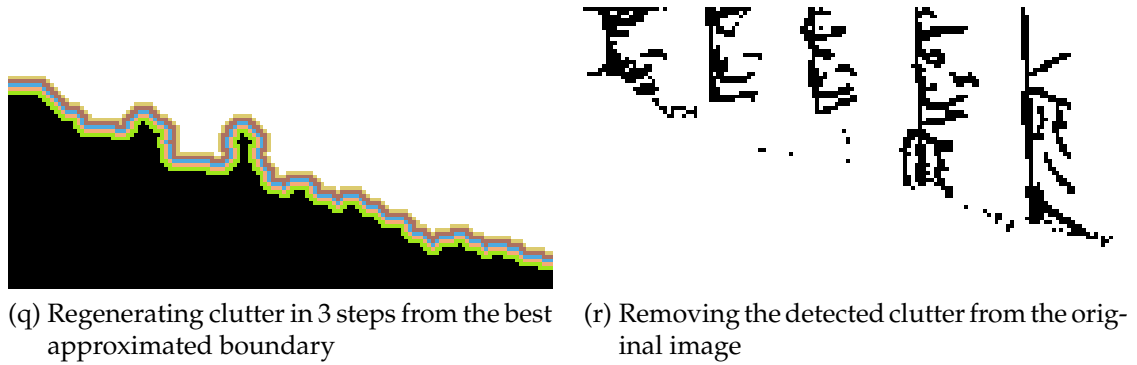
Figure 2.12: Clutter Removal Process.
