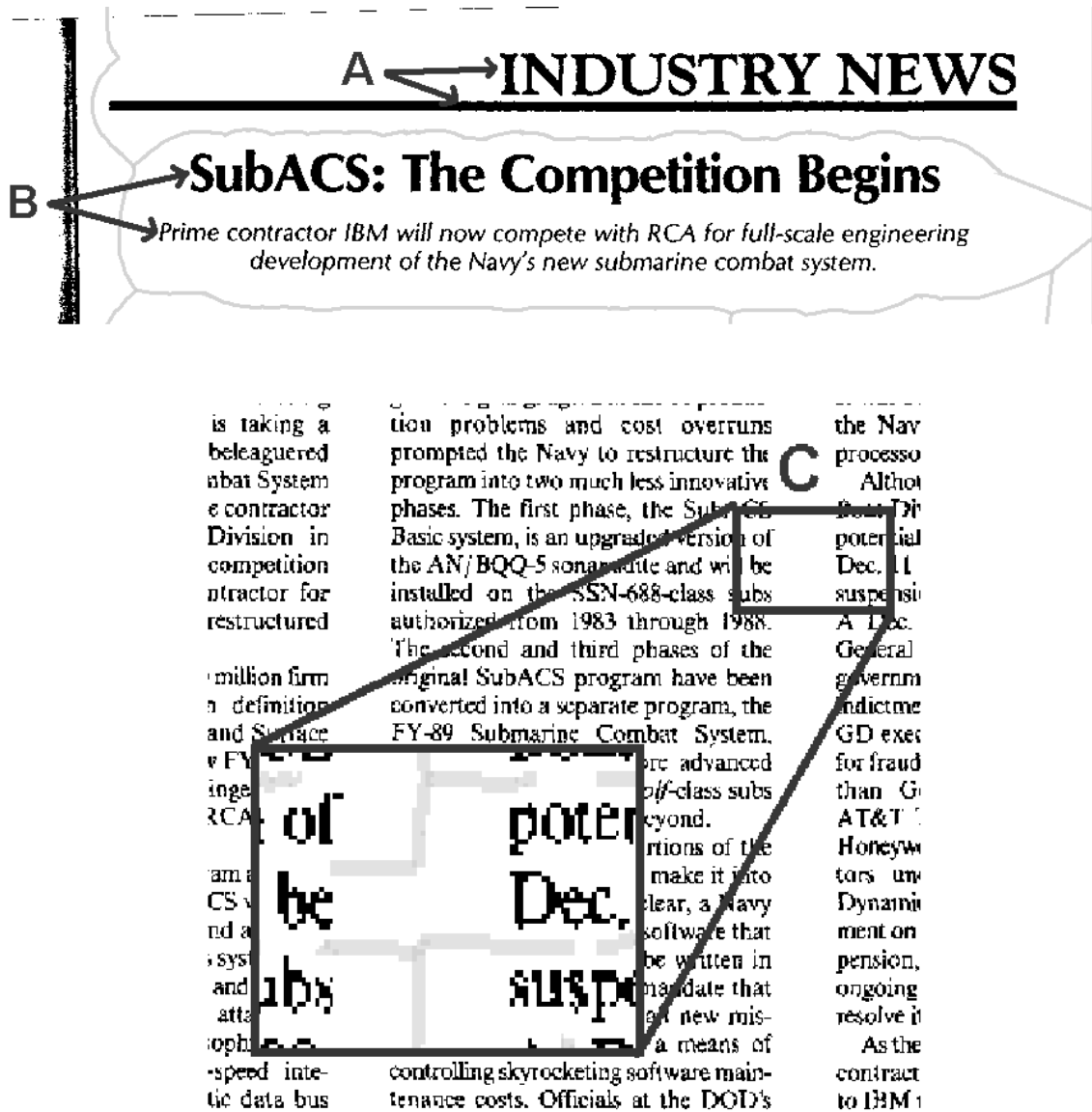
Figure 3.14: A and B depict increase in T_{d2} based on larger components, due to which dissimilar zones have been merged together. C depicts large components formed due to touching-characters ( be , Dec ). This in turn increases T_{d2} and removes the edge, leading to the fusion of two columns into a single zone.
