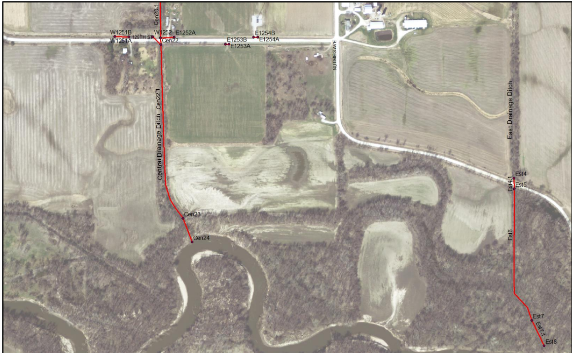
Figure G-1: Links and Nodes for the Downstream Ends of the Central Drainage Ditch and the East Drainage Ditch
