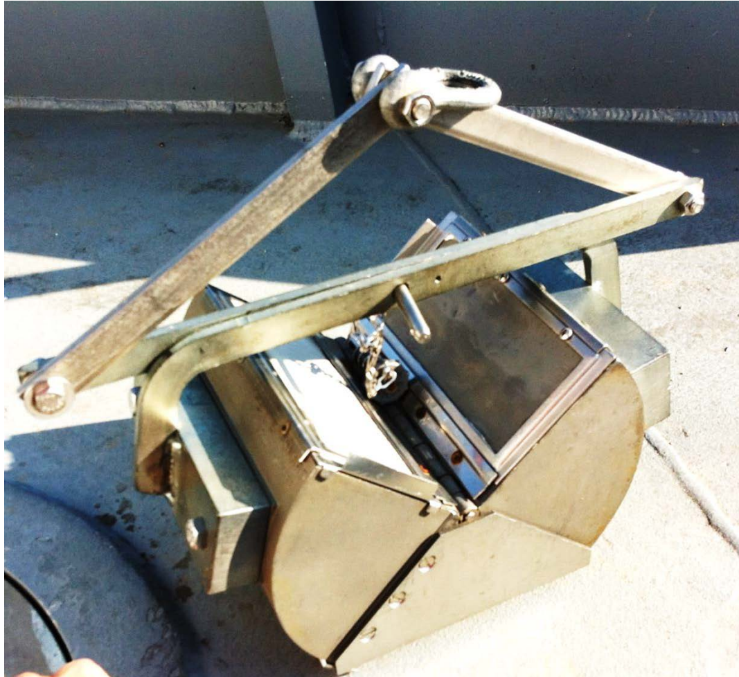
Figure 2-2. The ponar, or Van Veen Grab Sampler, was used for sampling surficial sediment.
