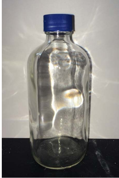
Figure 2-7. ASE collection bottles. Collection bottles were triple rinsed with methanol, hexanes, and acetone. Caps were triple rinsed and housed a Teflon lined septa which was replaced before each use.
