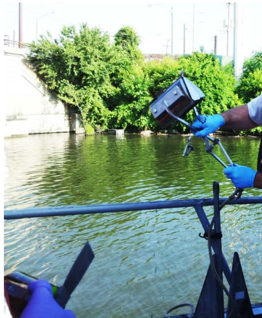
Figure 2-3. Retrieving the ponar.
